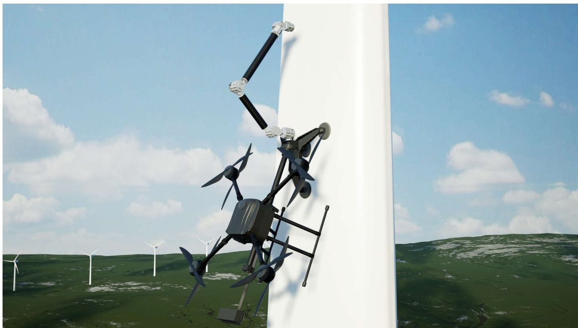
Figure 3.1 UAV perched on a wind turbine blade with the NRC’s Base Attachment Module and deploying a robotic arm
