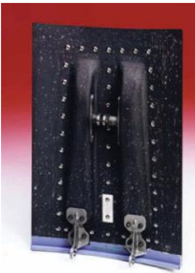
Figure 2-8 Volet de tuyère C/SiC SEPCARBINOX [25]
