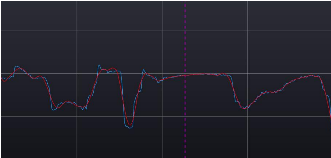
Figure 4.6. Savitzky Golay filter for acceleration pedal channel
