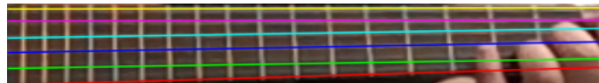
Figure 4.17 Image showing the detected fretboard strings with color-coding. The color codes are as follows: red for the first string, green for the second string, blue for the third string, cyan for the fourth string, magenta for the fifth string and yellow for the sixth string.
