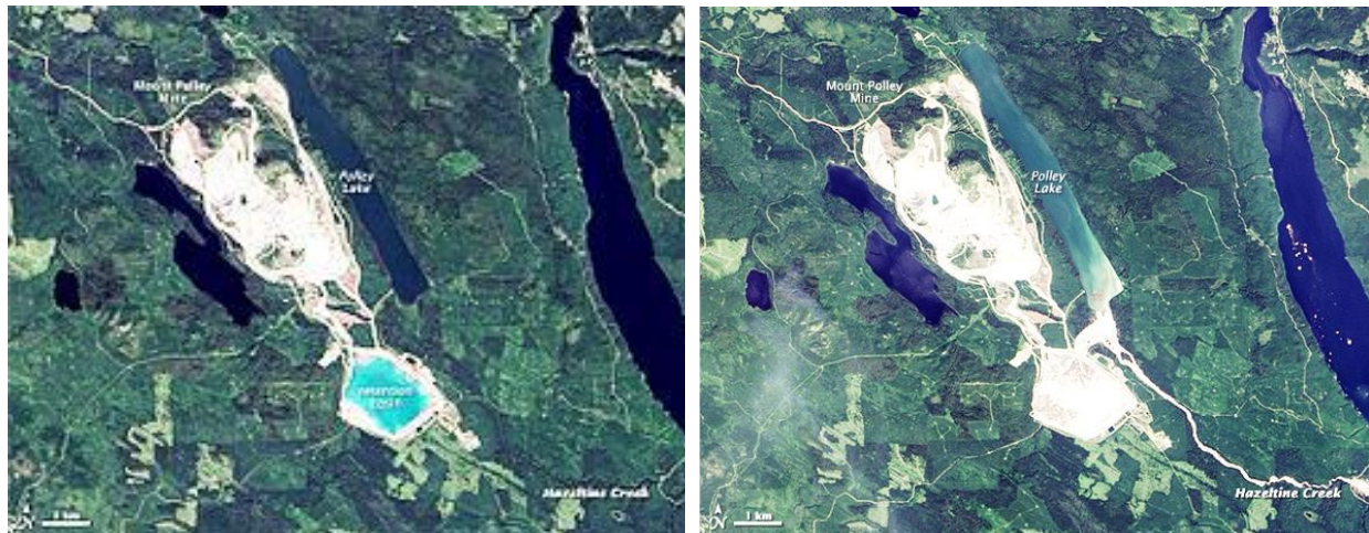
Figure 2.2 satellite image of Mount Polley before (left image) and after (right image) the tailings dam breach (Mahdi et al., 2020)
