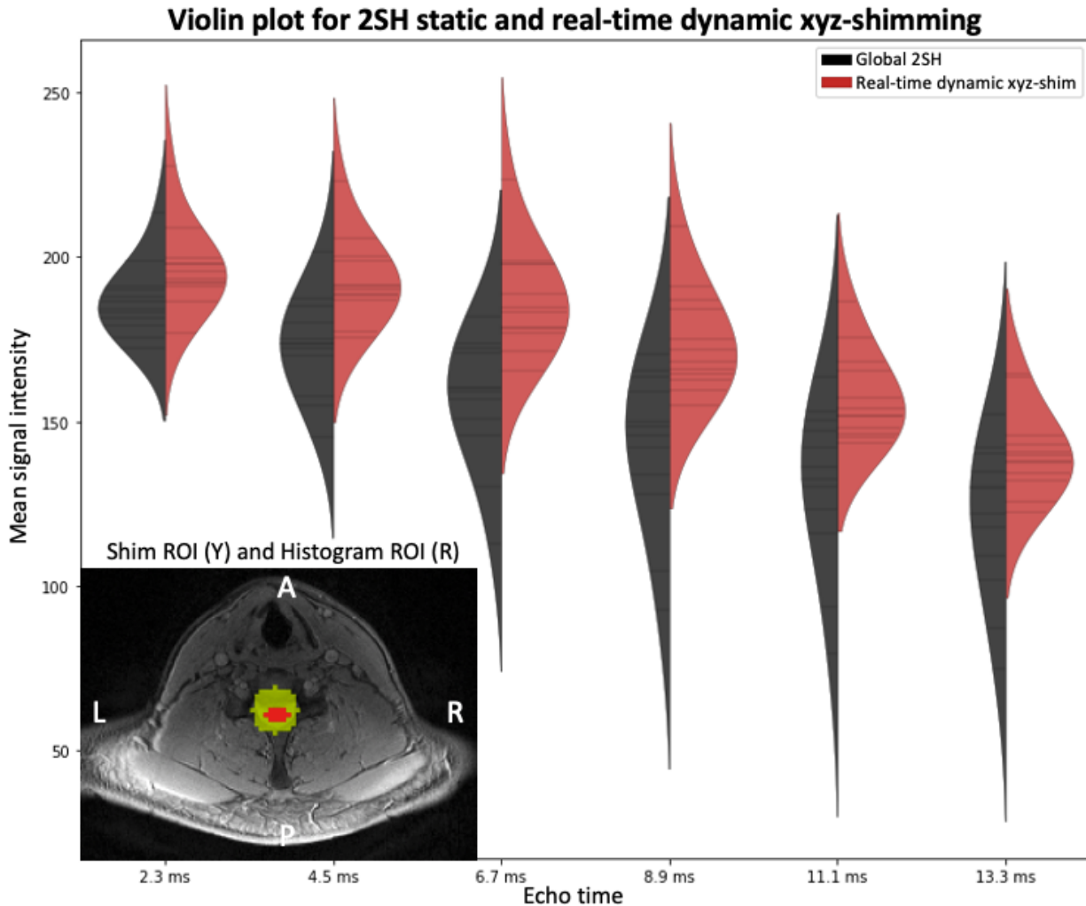
Figure 4.9: Violin plot comparing the signal distribution within the spinal cord with 2 nd order global shimming (black) and with real-time dynamic xyz-shimming (red) for multiple echo times. Mean signal intensity across slices and echo times: global/real-time: 151.54/174.99. Average standard deviation within slices: global/real-time: 19.61/13.81. An axial slice showing the location of the shim ROI for real-time shimming as well as the segmented spinal cord is shown at the bottom left of the plot.
