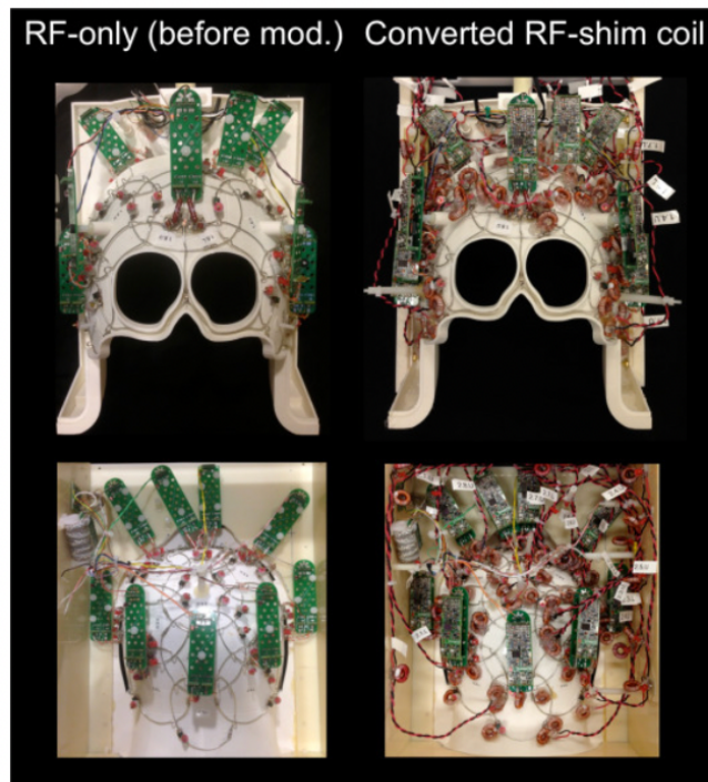
Figure 2.12: Top and bottom halves of coil before and after conversion to a combined RF-shim array. From [12].
