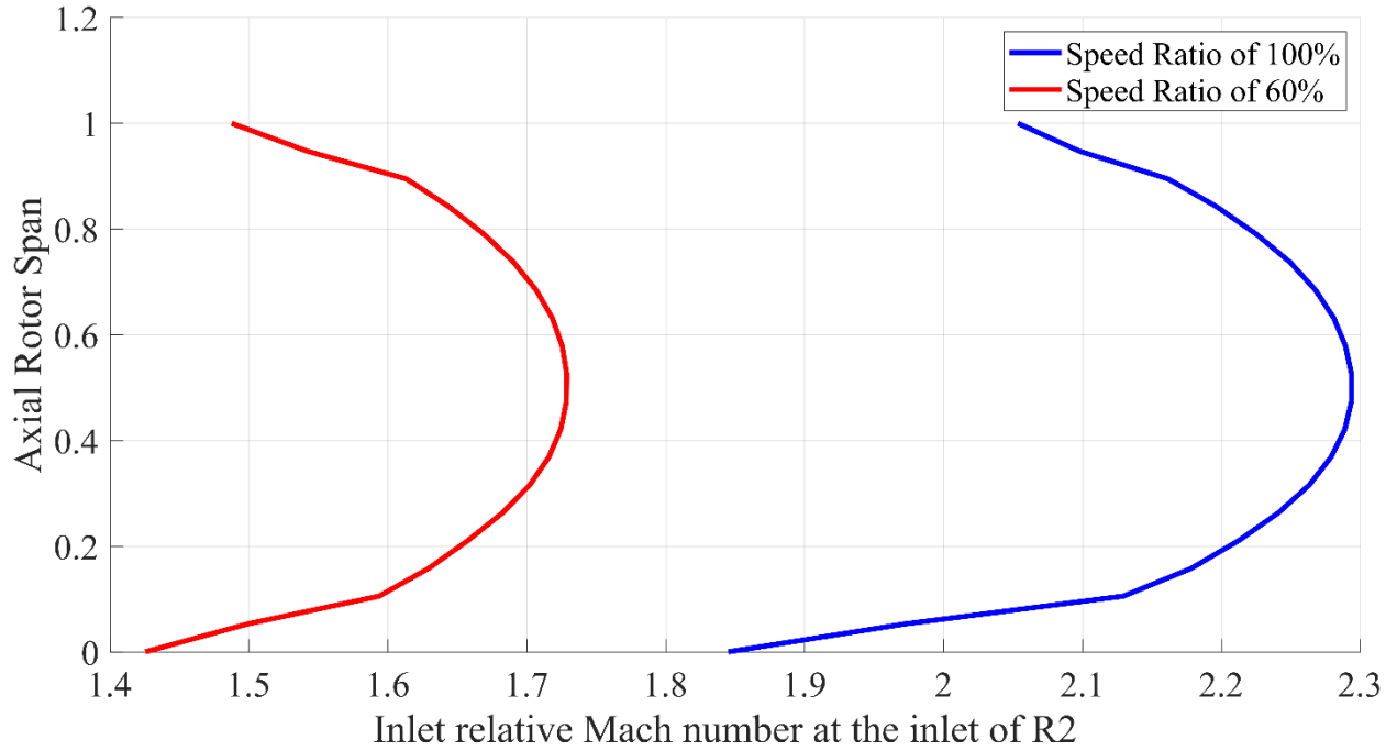
Figure 5-4 Spanwise distributions of relative inlet Mach number for axial rotor
