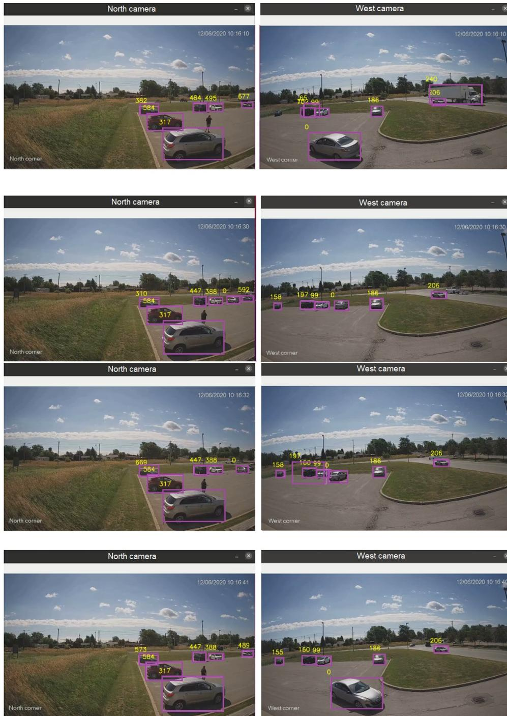
Figure 4.9 Sample results on Cysca's test videos. The three scenes are captured in about 450 frame span. In the first scene. There is vehicles#0 that enters the parking lot. In the second scene the vehicle is parked having the same global IDs in both cameras. In the third and fourth scene we can see this vehicle that starts moving again and exits the parking lot while it keeps the same global ID 0.
