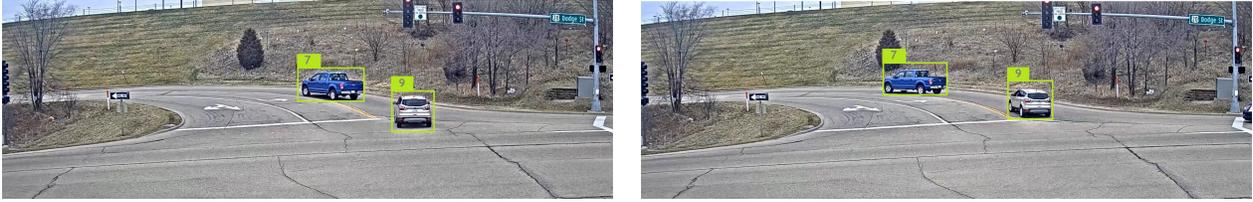
Figure 2.1 Sample frames of output of a SCT. The two scenes are captured in about 400 frame span. In both scenes two vehicles are located in the images, rounded by a bounding box, and assigned to consistent IDs (the white car is assigned to ID no.9, and the blue car is assigned to ID no.7).
