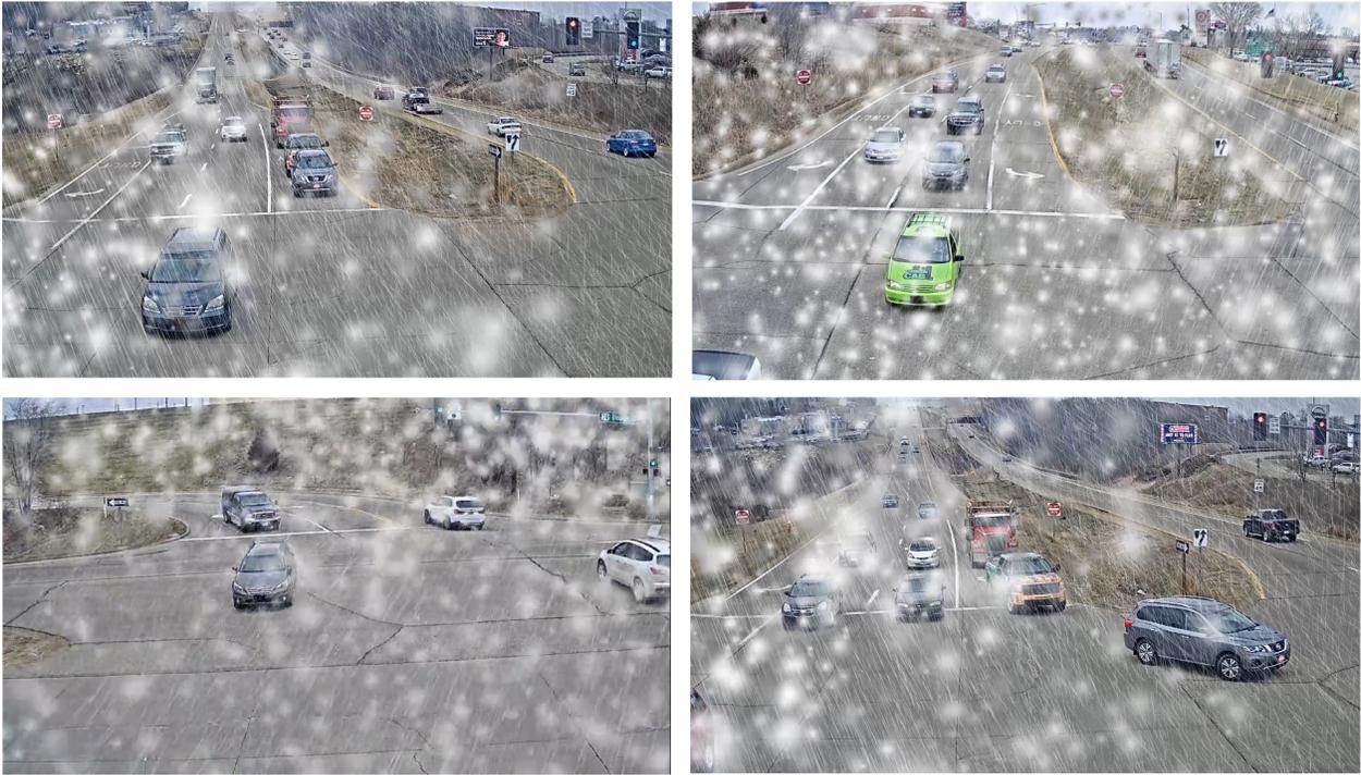
Figure Figure 4.2 Example frames of the created synthetic dataset based on AIC20 benchmark, containing snow, rain and wind effects.
