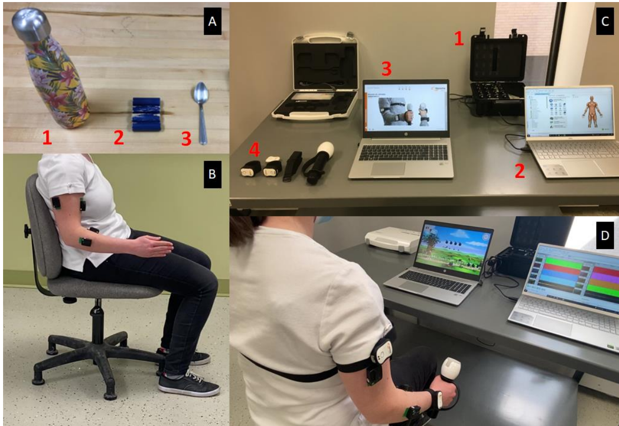
Figure 5-2. Measurement session – A. The three objects used for functional gesture: bottle (1), four wood cylinders (2), spoon (3). The door used for the fourth functional gesture was not represented. B. Neutral position for discrete gesture recording. C. Material needed for Armeo@Senso recording: Trigno (Delsys) base station and EMG-IMU sensors (1), EmgWorks (Delsys) software (2), Armeo@Senso software (3), wearable Armeo@Senso IMU sensors (4). D. Subject playing with Armeo@Senso High Flyer (shoulder) game during session.
