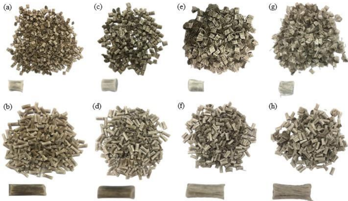
Figure 5.5: LFT pellets obtained with two different lengths (6 mm and 15 mm) and four different void contents. The top four images represent the 6 mm LFT pellets and the lower four images represent the 15m LFT Pellets. (a) & (b) 4%, (c) & (d) %8, (e) & (f) 15% and (g) & (h) 22% void content. Pelletizing pultrudates with void contents above 8% seems to result in cracked and opened pellets.
