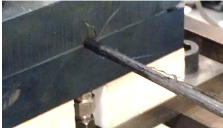
Figure 4.9 Image of the cooling die's exit during PEI-300 experiment. The image is displaying dry carbon fibers detaching from the pultruded material upon exiting the cooling die. This is a typical sloughing event.
