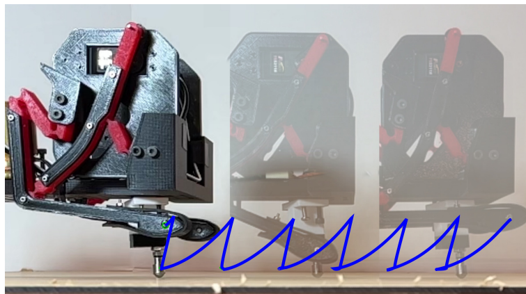
Figure 4.15 Composite picture of five steps with the recorded foot trajectory (the robot is moving from left to right)
