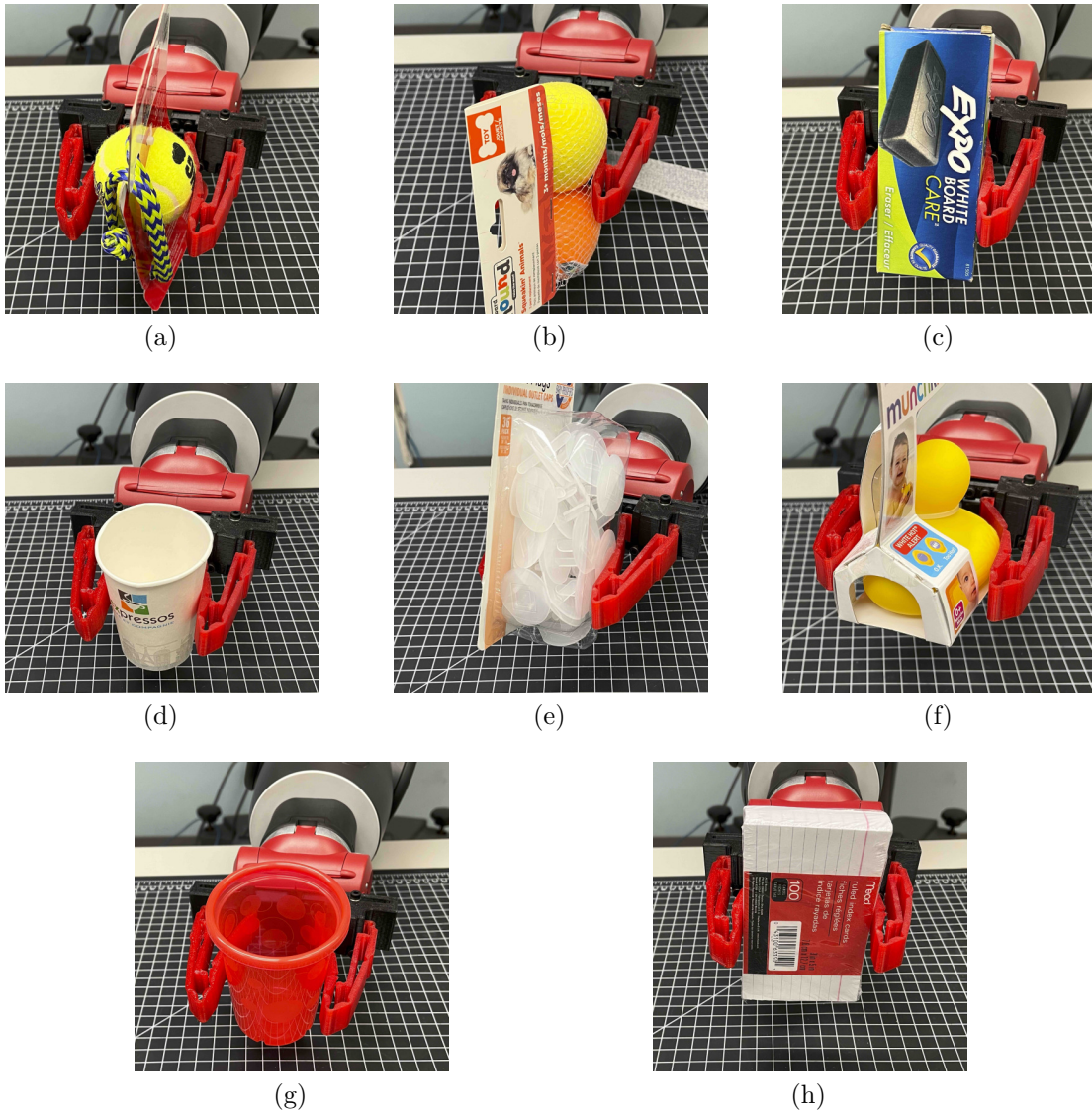
Figure 5.18 Grasps of various objects from the 2016 Amazon picking challenge in low-stiffness mode.
