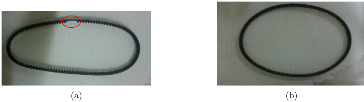
Figure C.3 G.U.N.T (PT 500.14) - the healthy and faulty belts
