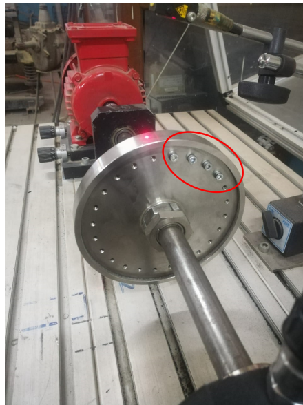
Figure C.4 G.U.N.T (PT 500.14) - presence of unbalanced weights
