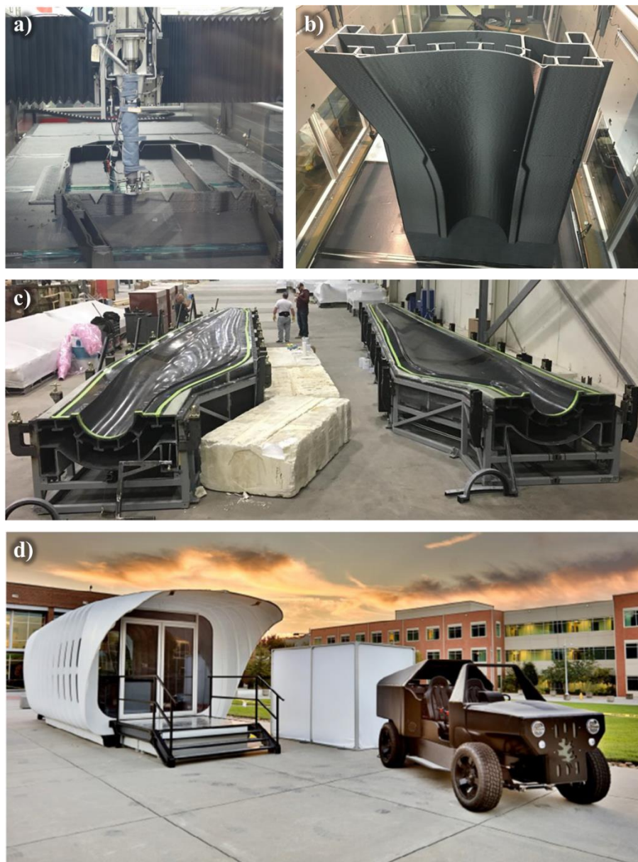
Figure 2-4: a) BAAM-CI system printing a vehicle frame [24] b) 1.8-meter-tall wind turbine blade mold segment printed on the BAAM-CI system [18] c) Completed two-part wind turbine mold after fiberglass application and machining [18] d) Single-room building and range-extended electric vehicle printed on the BAAM-CI system [24]
