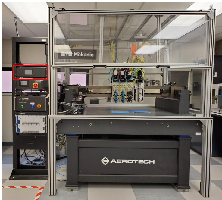
Figure 5-4: Printhead controller installed in the rack beside the Aerotech system enclosure
