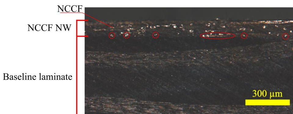
Figure 4.8: NS0.1 cross-section observation with optical microscope ( \times 90 ). Circled in red: NCCF in contact with the first carbon fibre ply.
