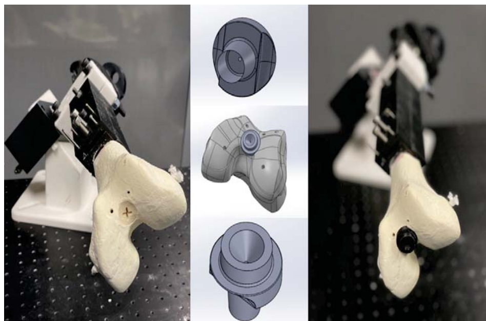
Figure 3.4 An illustration of the placement of the MAEP on the distal femur bone (anatomical landmark of the sawbone)
