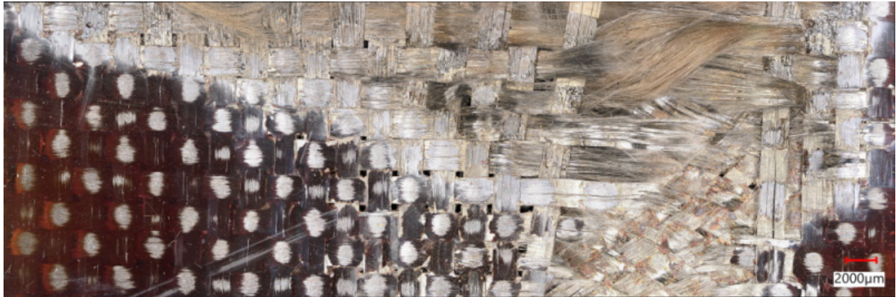
Figure 3.13 Backside of a CF epoxy sample strip exposed for 15 s to a calibrated propane flame and tensile-tested afterwards.
