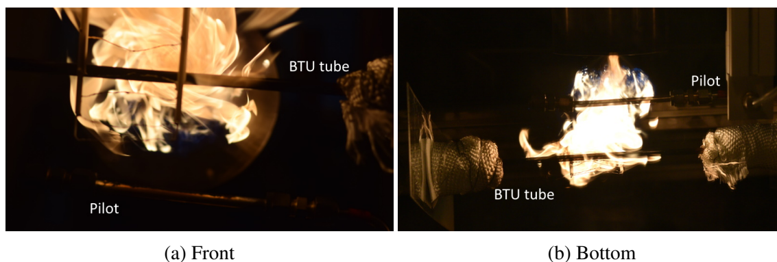
Figure 3.6 (a) Front view showing the flame cross section perpendicular to its axis and (b) bottom view revealing the flame width at the tube location, imaged through the mirror. The flame shown corresponds to approx. 8 kW. Burner operating parameters: 3 g/s air and 0.19 g/s jet-fuel.
