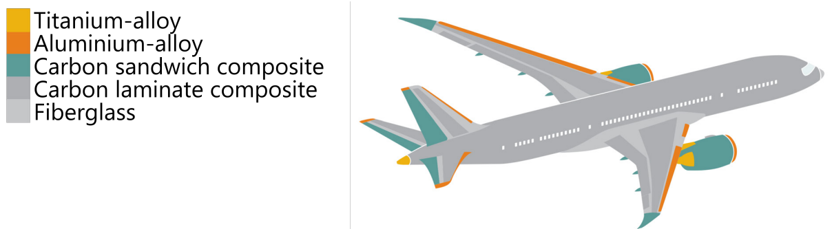
Figure 1.1 Usage of materials in the Boeing 787. Air-frame and primary structures are comprised half of carbon fibre reinforced plastic and other composites. Reprinted with permission from [3]. Copyright 2016 The Boeing Company.
