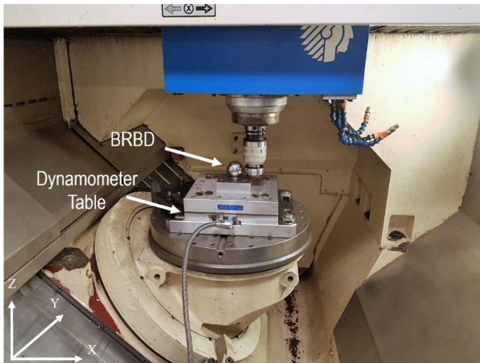
Figure 6.6. Installed dynamometer table and BRBD device on the machine tool.
