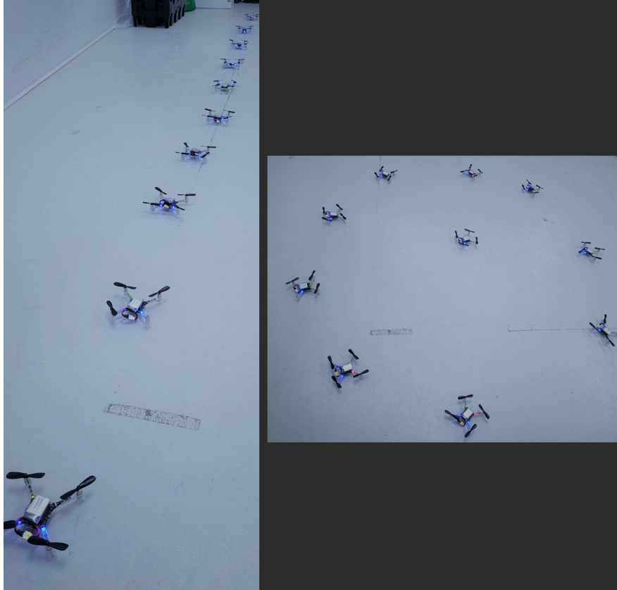
Figure 4.6 Configurations used for consensus tests. Left: chain like configuration; right: circle-like configuration
