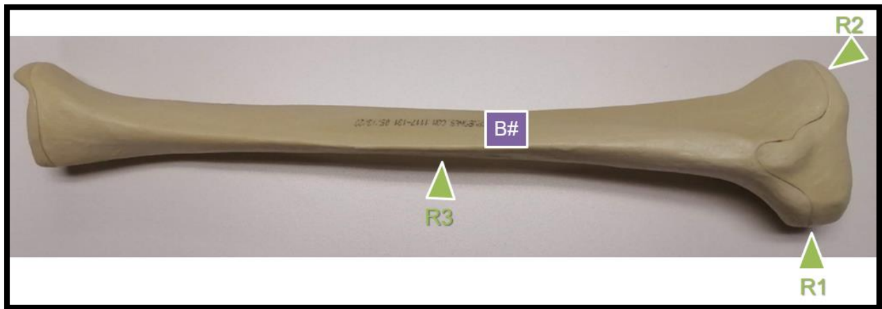
Figure 4.1 Placement of the divots on the sawbone.
