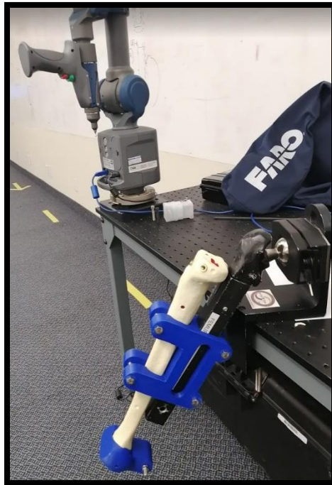
Figure 4.2 The sawbone and FARO arm are installed on the table.
