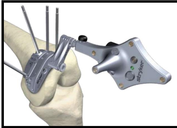
Figure 2.12 The Stryker Femur/Tibia tracker (Stryker, 2007a).
