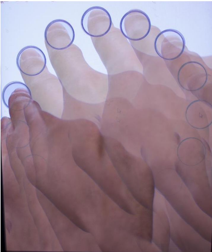
Figure 3.44 – Composite image made by combining 15 images with the index finger touching each of the 15 targets. As can be seen, the bottom targets tend to be obscured, while the top targets are more visible.
