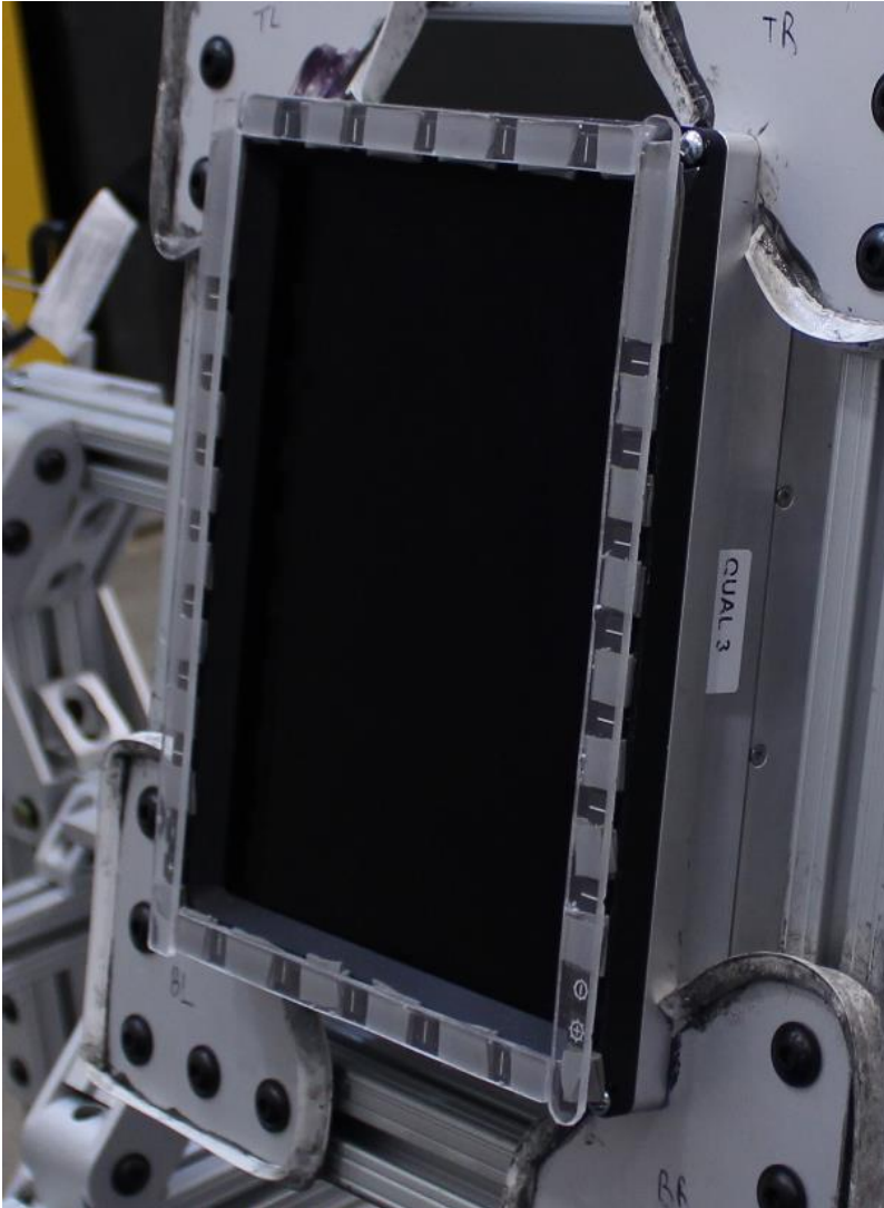
Figure 3.58 – A barrier was affixed to the bezel, in order to cover the bezel keys, to prevent them from being accidentally activated in the hand-support condition.
