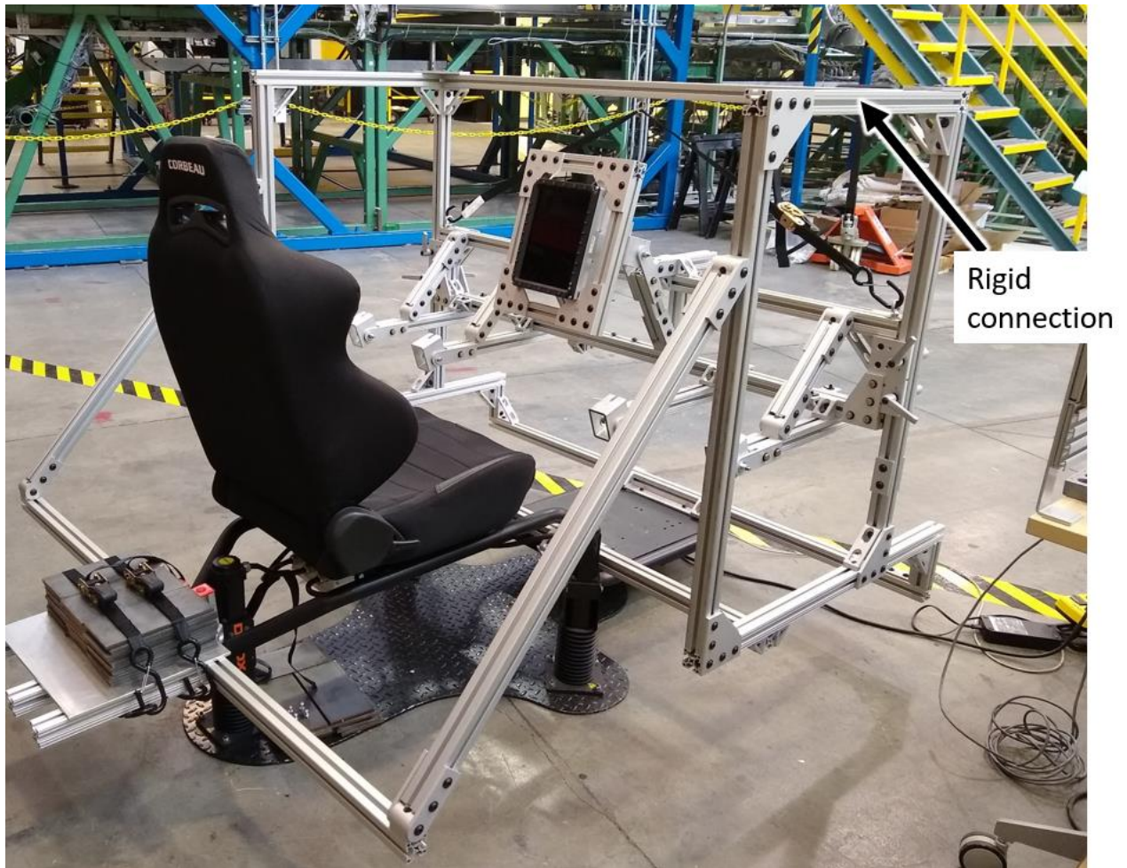
Figure E.3 - The first version of the structure, which had the screen support columns connected rigidly, on top, with the rest of the structure.
