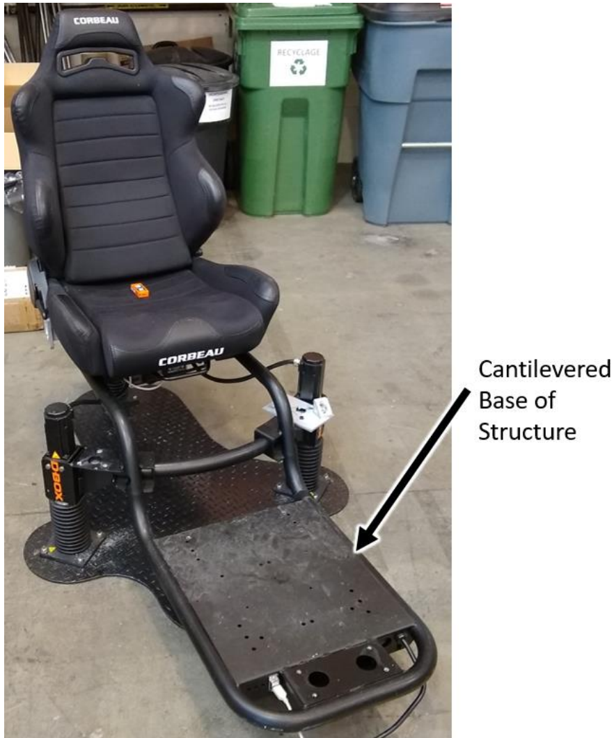
Figure E.1 – The front section of the structure is cantilevered out beyond the motors, and flexes during vibration.
