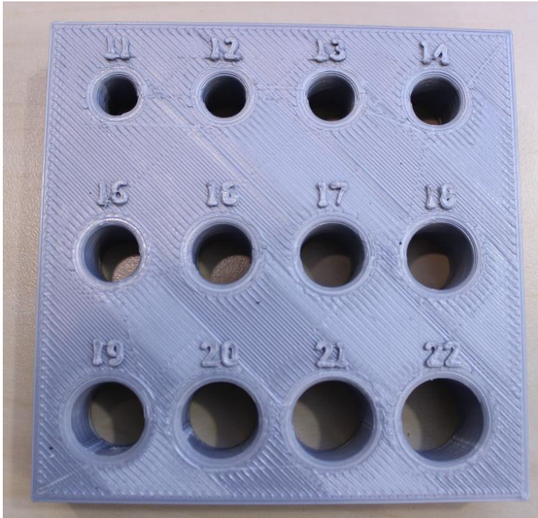
Figure 2.32 – The 3D printed block used to measure participants' index finger widths.
