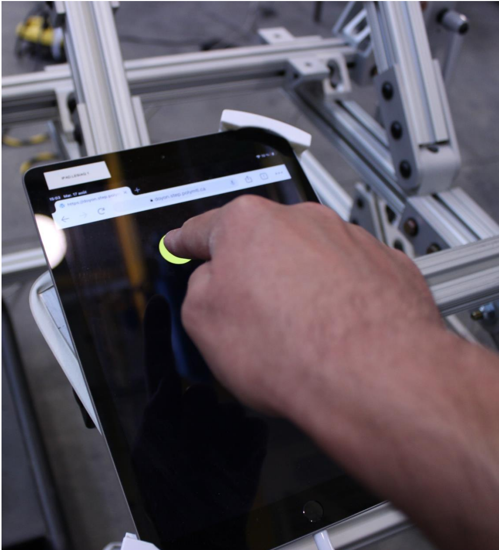
Figure 2.20 – Image of the Fitts' selection task website programmed by Philippe Doyon-Poulin. Only one target location is shown at a time. The active target is shown as a yellow circle on a black background.
