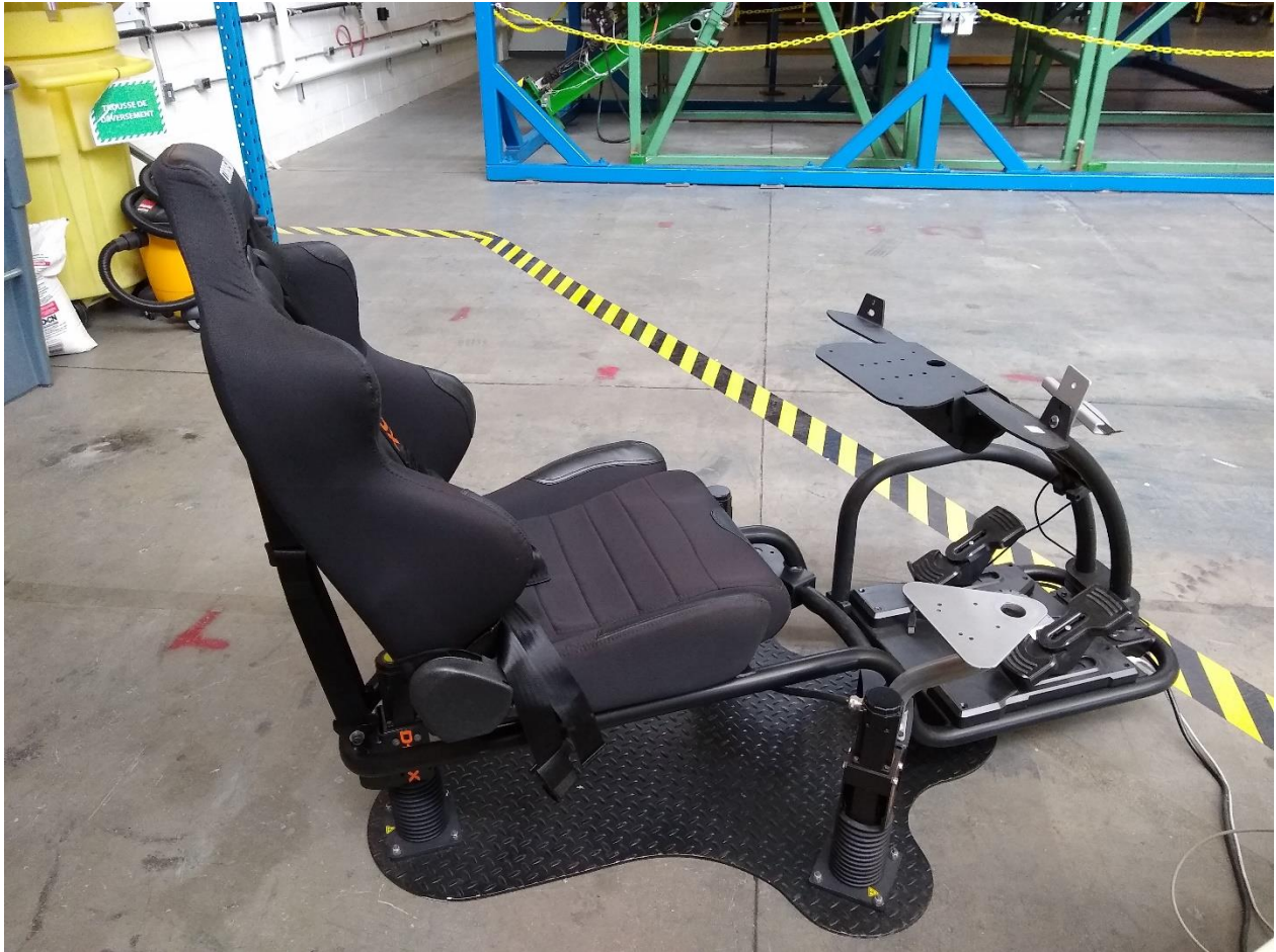
Figure 2.12 - Image of the D-Box GP Pro 500, before the test structure was built onto it.
