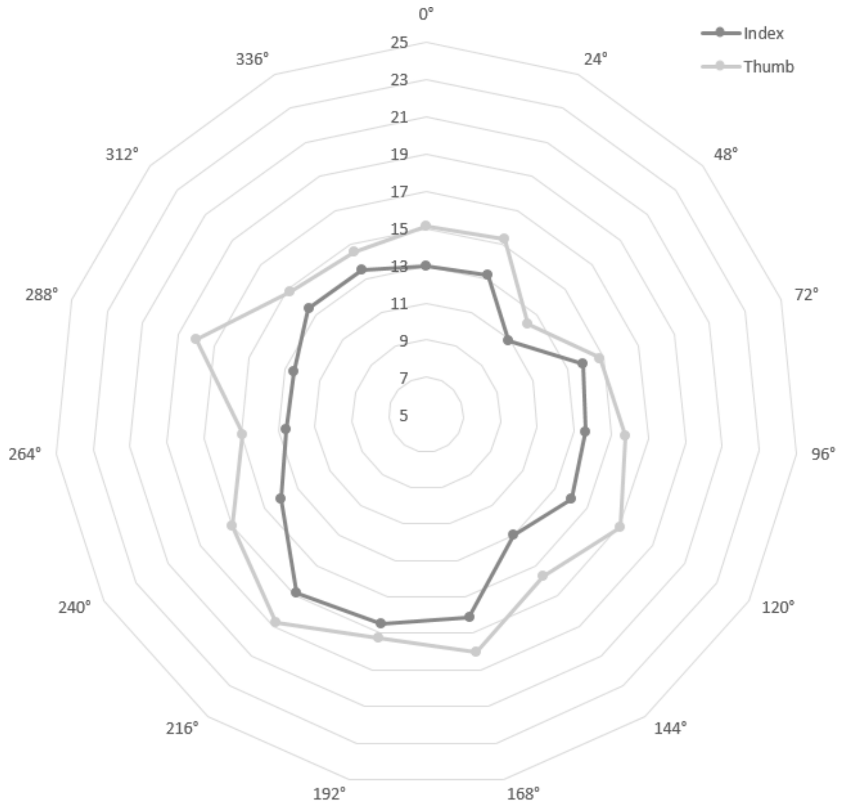
Figure 3.36 – Percent error rate versus selection angle, for the index finger and thumb conditions. The large screen and small MCDU screen have been excluded from this average, as well as any participants that used their left-hands. Note that any increase in error rate at 192°, 288°, 24° and/or 120 may be partially due to order effects.
