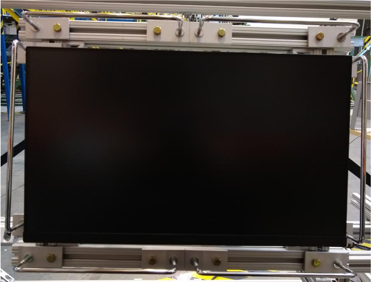
Figure B.1 – Drawer pull handles surrounding the large touch monitor. We initially planned to use these as hand supports.
