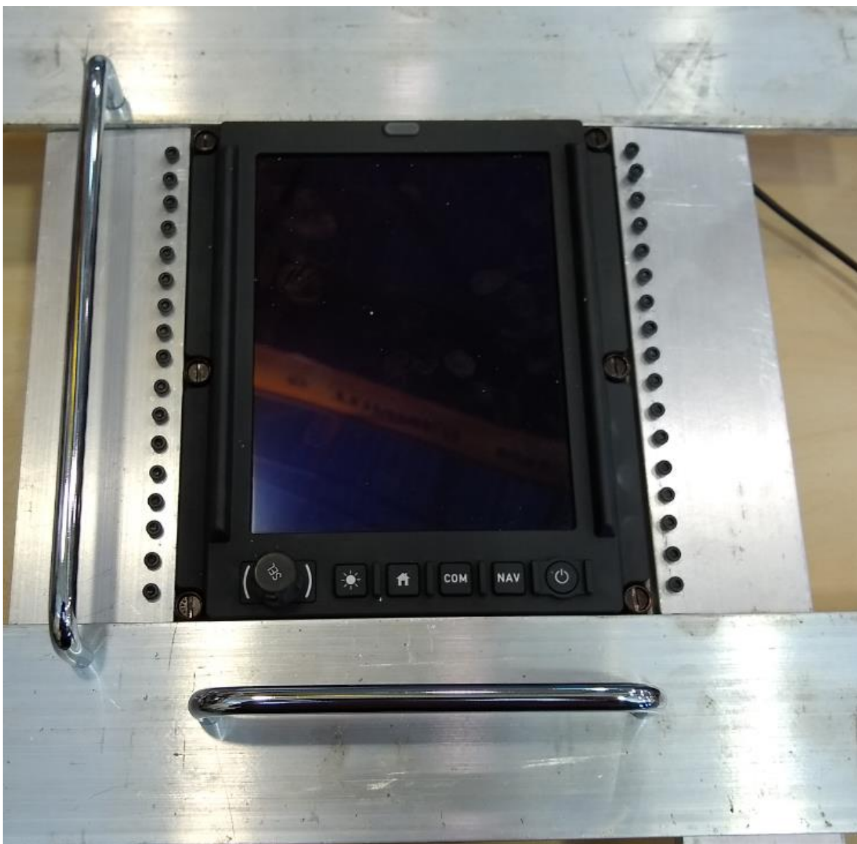
Figure B.3 – Proposed placement of the drawer pull handles around the small screen. This image just shows two handles, placed to the left and bottom of the screen, but there would have also been handles placed to the right and top, as well. None of these handles were ever installed.
