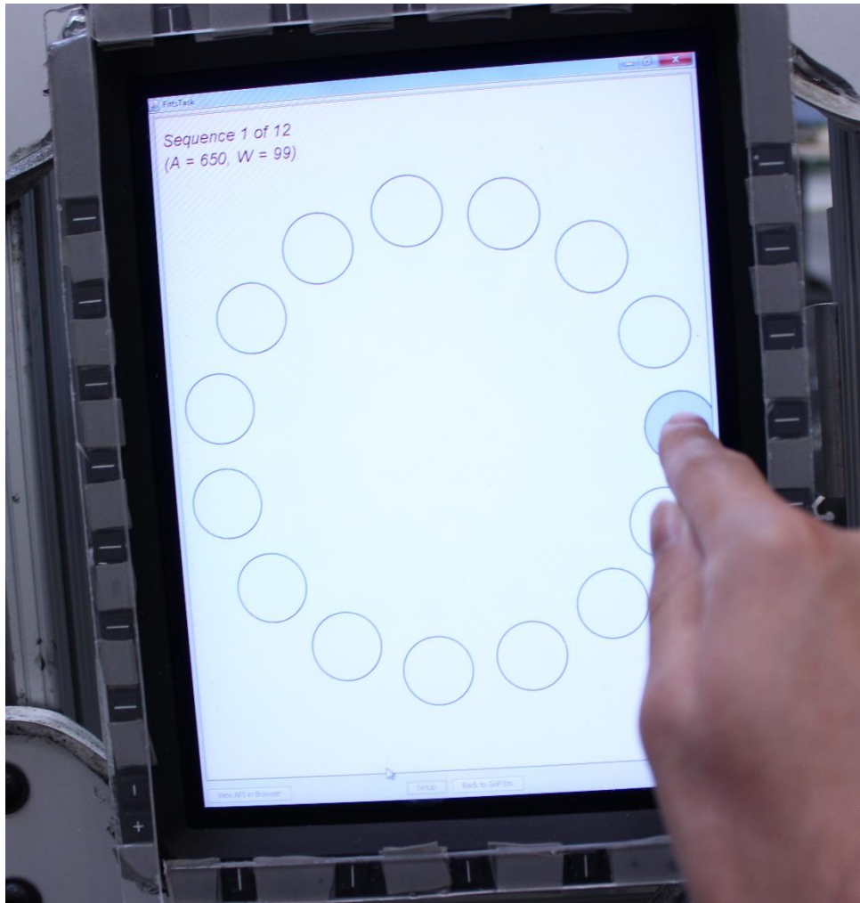
Figure 2.19 - An image of the MFD screen running MacKenzie's GoFitts software application.
