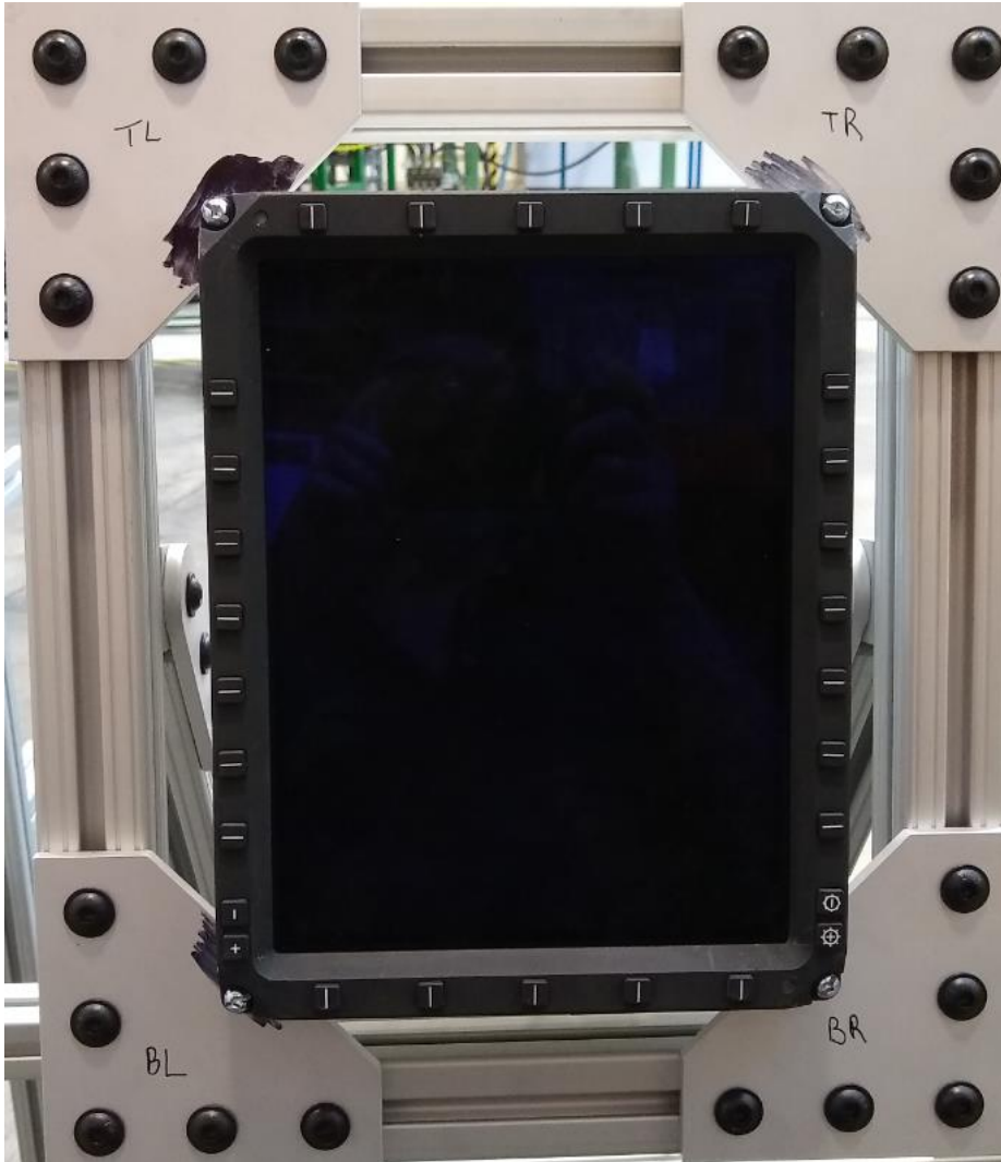
Figure 3.57 – When using the bezel edge as a hand support, the protruding bezel keys of the MFD screen were accidentally clicked, on several occasions, while reaching for a target.
