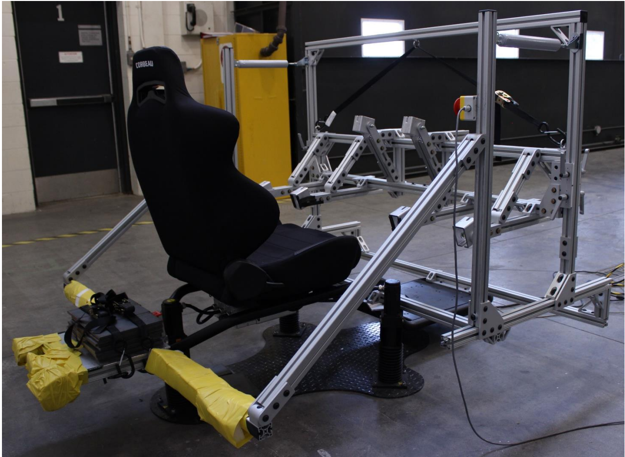
Figure 2.13 - D-Box GP Pro 500 with test structure built onto it.
