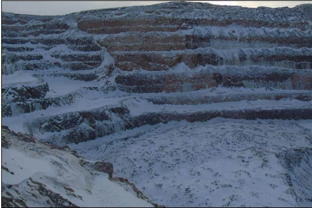
Figure 4.1 Blasted material at the foot of the highwall
