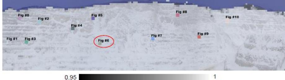
b) Deformation image: 24 hours after the blast
