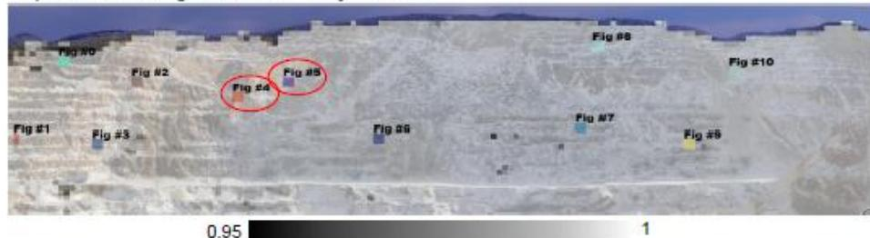
b) Deformation image: 24 hours after the blast
