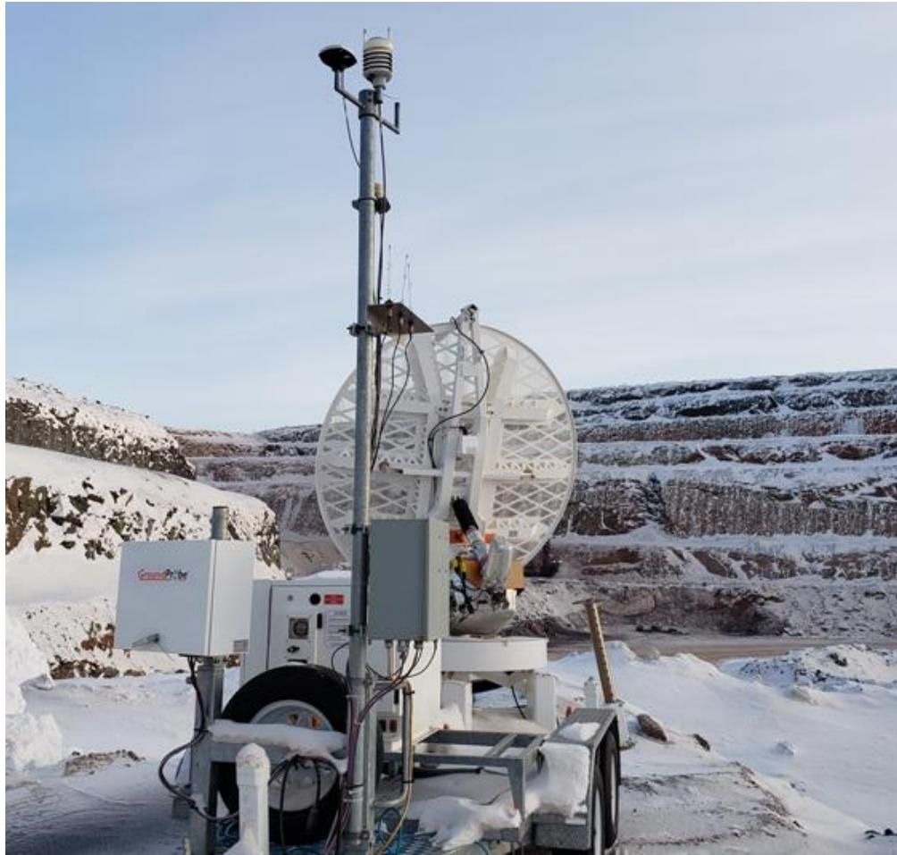
Figure 7.23 Slope Stability Radar monitoring the southeast wall
