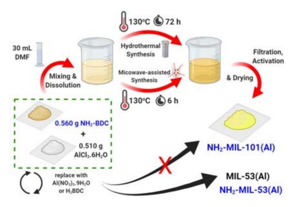
Figure 4.10 Synthesis of the amino-functionalized aluminum isomorph expressing color change between the different steps.
