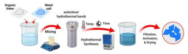
Figure 2.8 Conventional hydrothermal/solvothermal method for MOF synthesis.
