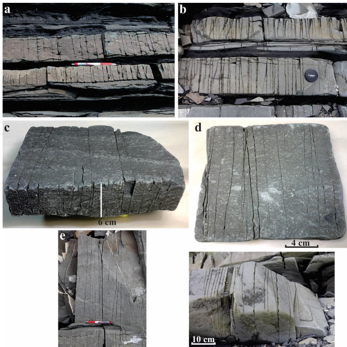
Figure 4.24 Examples of jointed calcareous greywacke beds with joint spacing to bed thickness ratio s/t \leq 0.2 but without cross joints developed as predicted by numerical models of Bai et al. (2002). Calcareous greywacke consisting of quartz, feldspar, calcite and clay has a positive Poisson's ratio (Ji et al., 2002). Samples collected from the External Humber Zone of the Appalachian orogen at Petite Vallée, Quebec, Canada (GPS coordinates 49.22133° N, 65.03569° W). (a-b) View from a plane perpendicular to the bedding surface and to the systematic joints. (c and f) Jointed sandstone resembling a sliced-up loaf of bread. (d-e) View from the bedding surface.
