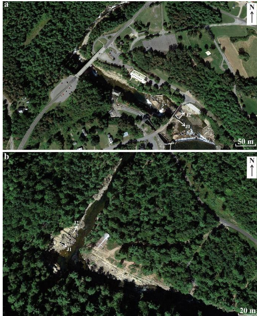
Figure 4.16 Orthogonal joints control on gorge orientation at Ausable Chasm (New York State, USA). The Ausable River makes a right-angle turn from the northwest direction (joint set J1) to a northeast direction (joint set J2) near the highway bridge (a) and the Whirlpool basin (b).
