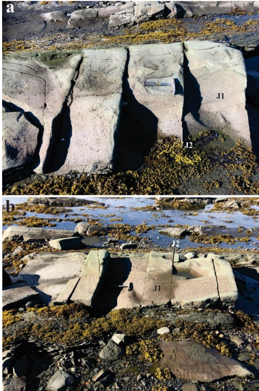
Figure 4.9 Steeply-dipping J2 joints observed on the J1 joint surfaces in thick sandstone layers. The joint spacing of J2 and particularly that of J1 are significantly smaller than the bed thickness.
