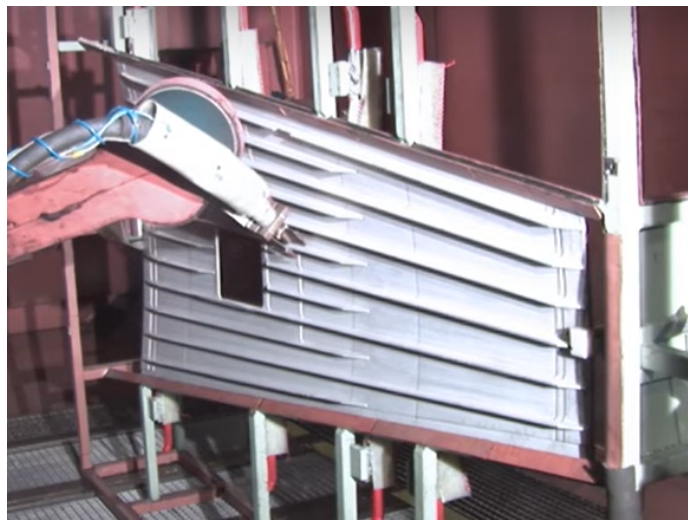
Figure 8.1 An integrally stiffened skin panel undergoing automated shot peening treatment. © KSA Kugelstrahlzentrum Aachen GmbH. Reproduced with permission.
