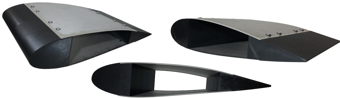
Figure 6.16 The model of an airplane wing skin shaped as the NACA 5430 airfoil with a chord length of 500mm. The upper and lower skins were shaped using the shot peen forming, and the forward and the back parts (black) were printed in 3D. The structure is assembled using binding barrels and screws.
