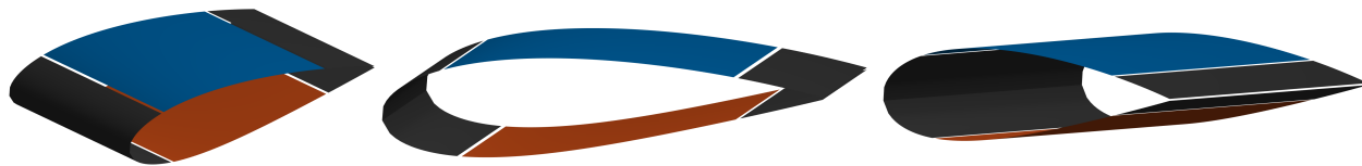
Figure 6.10 The two target shapes for the 320 \times 320 mm sized panels made of aluminum 2024-T3. The target shapes constituted parts of the upper (blue) and lower (orange) airplane wing skins. The wing was shaped as the NACA 5430 airfoil with the chord length of 500 mm.
