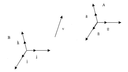
Figure 1: Relation between the measures  $[\underline{v}]_A$ ,  $[\underline{v}]_B$  of a given vector.
