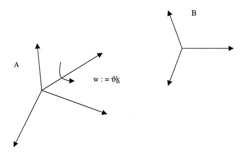
Figure 1: Euler's vector: the orientation of B is obtained by rotating A of an angle  $\vartheta$  (counter clockwise) about <u>k</u>
