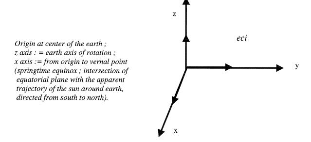
Figure 2: eci: Earth-centered inertial frame Reference frame
