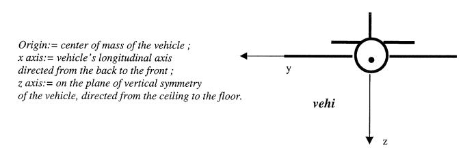
Figure 4: Reference frame attached to the vehicle
