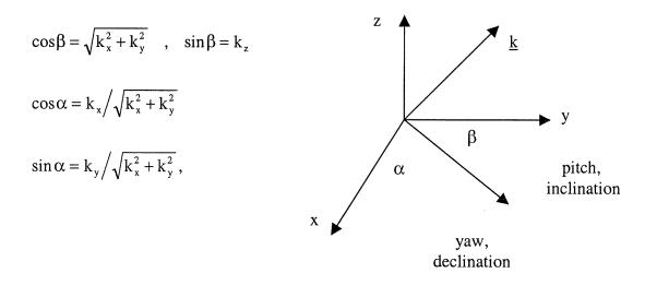
Figure 3 : Pitch and yaw angles of a vector relative to a frame.
