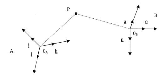
Figure 2: Measure of the position of a point with respect to a frame
