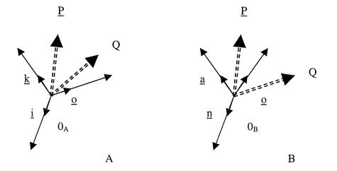
Figure 1: From the position of frames A and B relative to the stars to the orientation and angular velocity of B relative to A.
