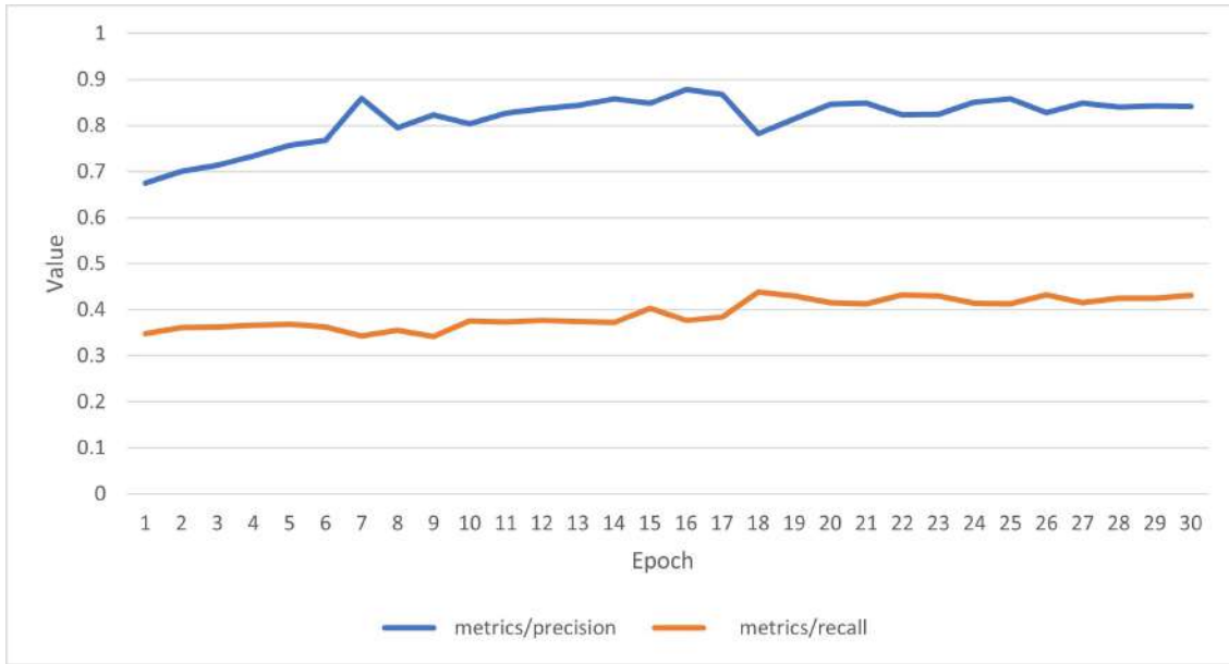
Figure 4.11 Precision and recall during fine-tuning of the preliminary network using the generated images
