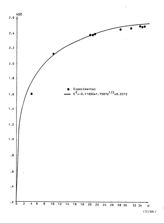
FIGURE 10: Calibration curve of the hot film 1231 AF-W (front sensor)
