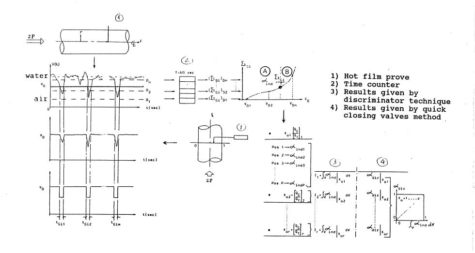
FIGURE 12: Calibration procedure of hot film for determining void fraction
