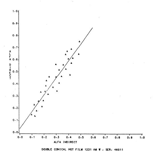
FIGURE 15: Calibration curve for void fraction
