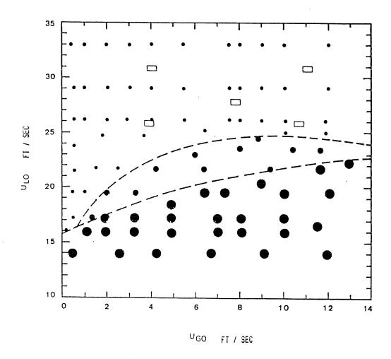
FIGURE 4: Flow map of horizontal air-water flow
