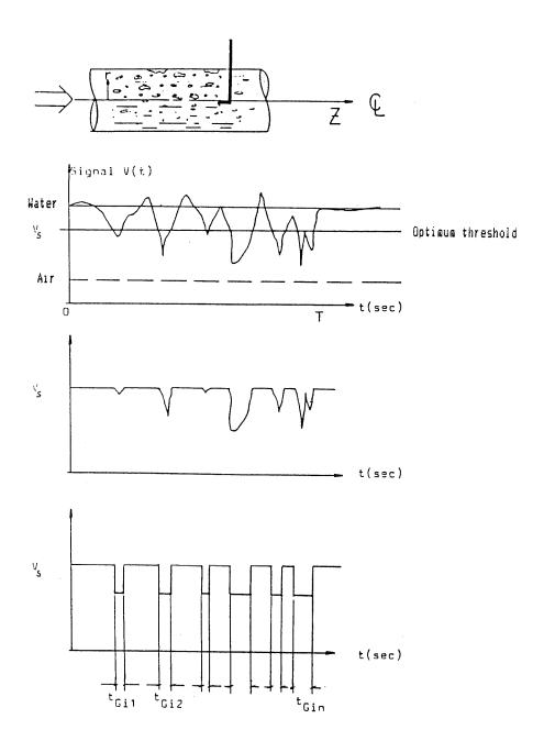
FIGURE 1: Local void fraction determined by discriminator technique with conditioned rectangular waves.
