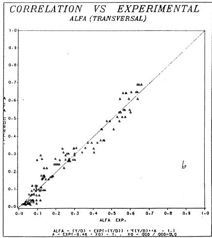
FIGURE 24: Comparison between experimental results and proposed void correlations in transversal plane
