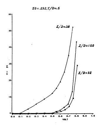
FIGURE 17: Average duration of bubbles obtained at optimum value of threshold level,  ${\rm optimum\ void} = \Sigma t_G/T\ ({\rm front\ sensor})\,.$
