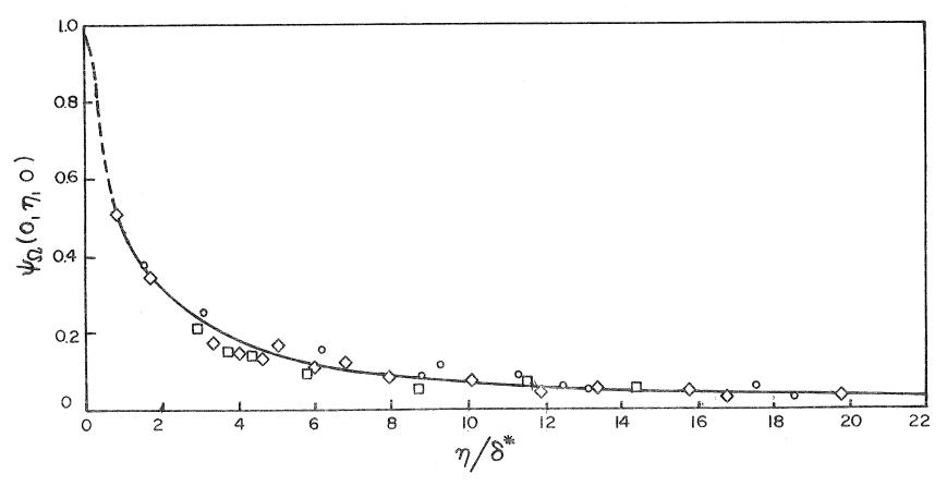
FIGURE 6b Lateral space correlation of the wall-pressure field,  $\Psi_{\Omega}$  (0, n, 0);  $\delta^{\star}is$  the boundary-layer thickness.
