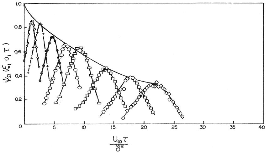
FIGURE 8 Frequency spectrum of wall-pressure fluctuations; where  $q_{\infty}$  is the free-stream pressure,  $\Omega$ , the central frequency;  $\delta^*$ , boundary-layer thickness and  $U_{\infty}$  is the centerline velocity. (Reproduced of Bull [36], Figure 7).
