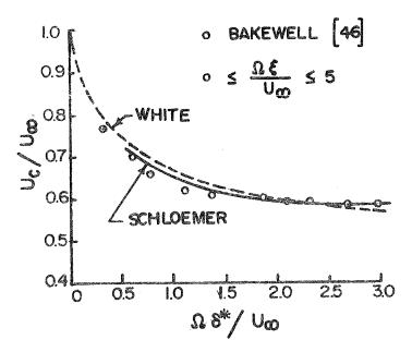
FIGURE 14 Convection velocity.
