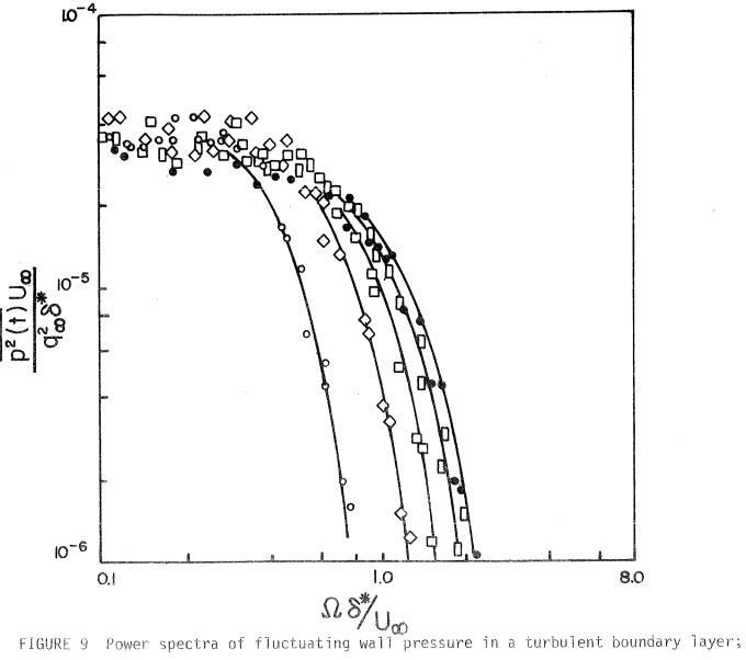
FIGURE 9 Power spectra of fluctuating wall pressure in a turbulent boundary layer;  $q_{\infty} \text{ is the free-stream pressure, } \Omega, \text{ the central frequency; } \delta^*, \text{ boundary-layer thickness and } U_{\infty} \text{ is the centerline velocity.}$
