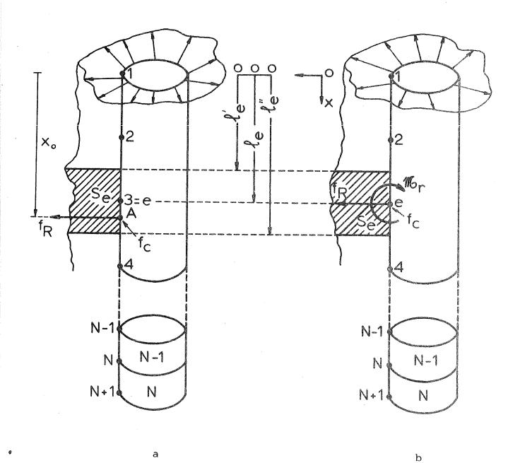
FIGURE 3 (a) Transformation of the continuous pressure field to a discrete force field
