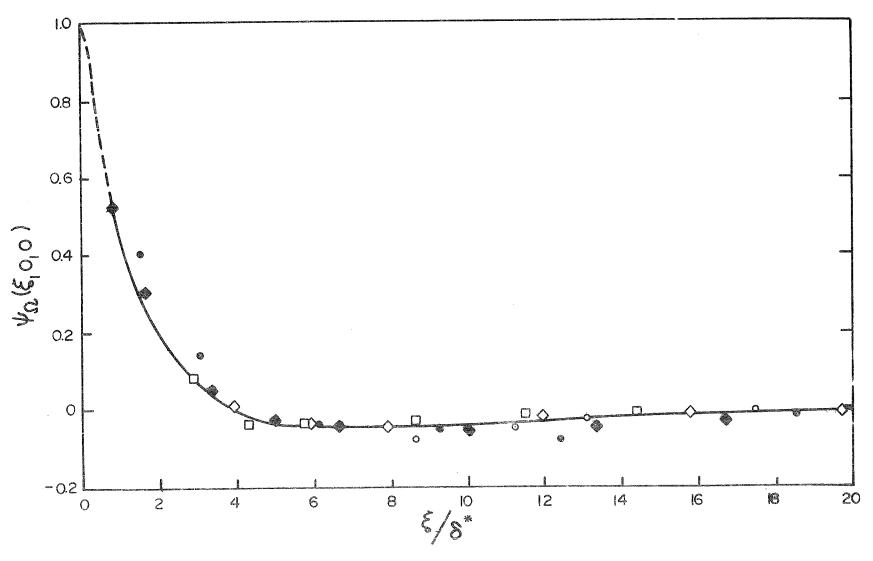
FIGURE 6a Longitudinal space correlation of the wall-pressure field,  $\Psi_{\Omega}$  ( $\xi$ , 0, 0) (Reproduced of Bull [36], Figure 9).
