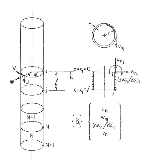
FIGURE 2 Definitions of the finite element used  $\text{and of the displacement vector } \delta _{\gamma} \text{ i.}$
