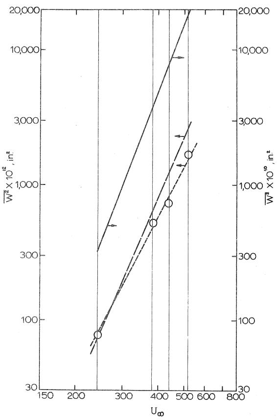
FIGURE 1 The mean square response of the radial displacement of a shell first studied by Clinch, as a function of the centerline velocity. -0--0- Clinch's experimental results for high-frequency response; — — theoretical results obtained by Lakis [12] (with n = 2 to n = 6) for high-frequency response (93 - 1,000 Hz); — 'total' response obtained by Lakis [12] (with n = 2 to n = 6).
