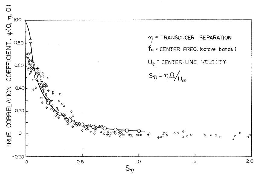
FIGURE 11 Lateral correlation versus Strouhal number based on centerline velocity. (Reproduction of Bakewell  $\begin{bmatrix} 46 \end{bmatrix}$ , Figure 30).
