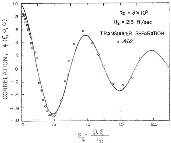
FIGURE 10 (Cont.) Longitudinal correlation versus Strouhal number based on convection velocity (U  $_{\rm CONV}$ ).
