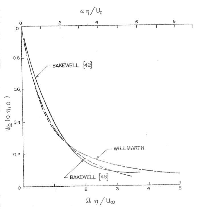
FIGURE 16 Magnitude of the lateral cross-spectral density. (Reproduced of Bakewell  $\begin{bmatrix} 42 \end{bmatrix}$ , Figure 9.
