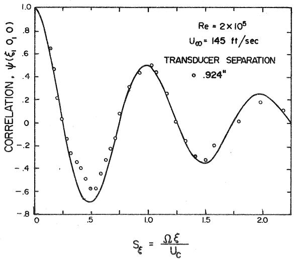
FIGURE 10 (Cont.) Longitudinal correlation versus Strouhal number based on convection velocity (U CONV).
