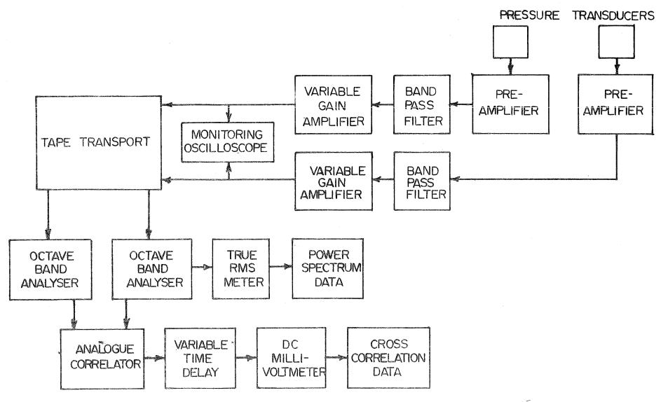
FIGURE 4 Block diagram of instrumentation used for recording and analyzing turbulent wall-pressure field.
