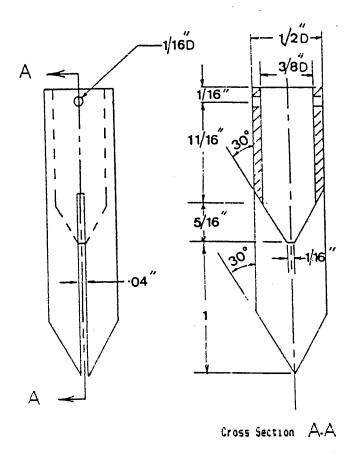
Figure 6.a Design of optimum liquid phase isolation
