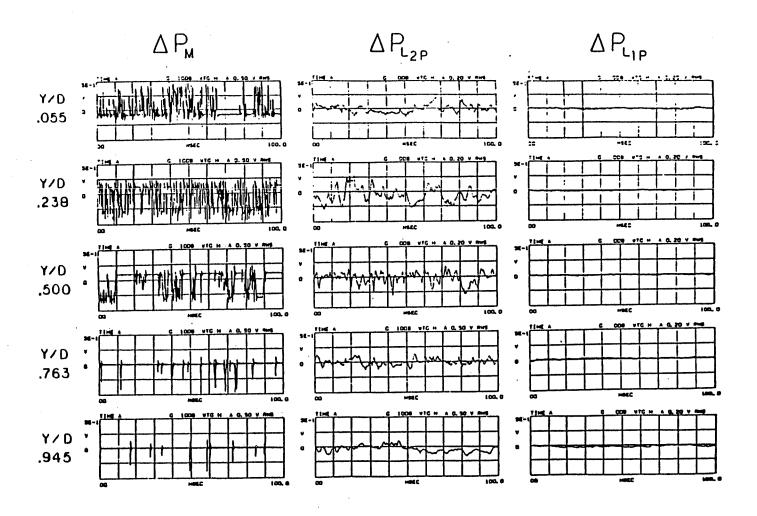
Figure 7.a Typical examples of dynamic pressure signals recorded at axial location 130D and  $X_{\rm o}=0.292$ .
