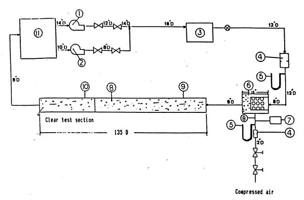
Fump (150 HP). 1) monitoring control valve 🔀 : regulator of constant pressure 2) Pump (75 HP). Closed pressure 3) manual control valve vessel (45 psi). 4) Orifice meter. 5) Hq U-manometer. 6) Air-Water mixer. 7) Pressure gauge. Thermometer. 8) 9) Test section. 10) Measurement apparatus (Pitot, probe...) 11) Open reservoir
