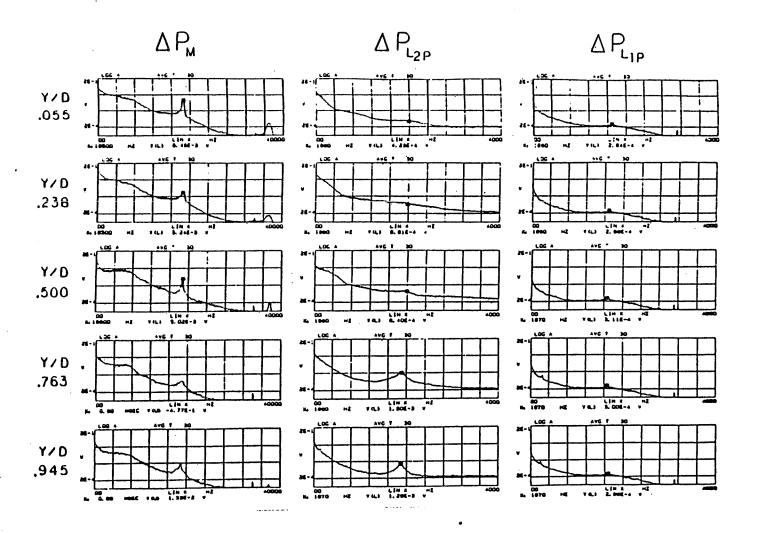
Figure 7.b Broadband frequency spectrum of dynamic pressure signals obtained in Figure 7.a.
