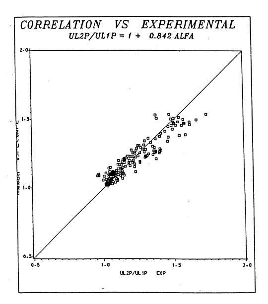
Figure 18 Comparison between values estimated by the proposed correlation and experimental results.
