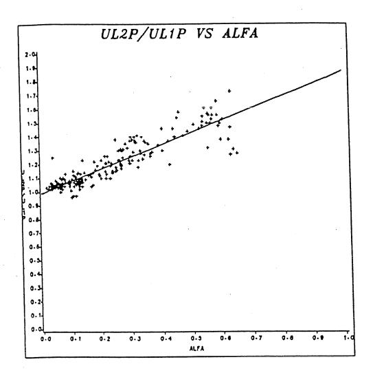
Figure 17 Variation of ratios  $U_{\text{LZP}}/U_{\text{LIP}}$  in terms of void fraction.
