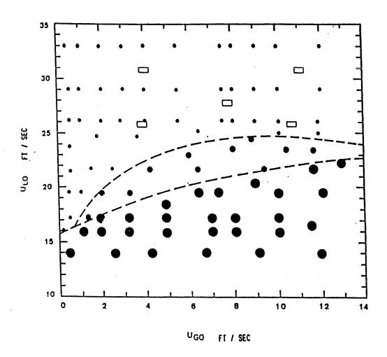
Flow map of horizontal air-water flow. (8-in. nominal diameter, fully developed flow z/D = 130)
