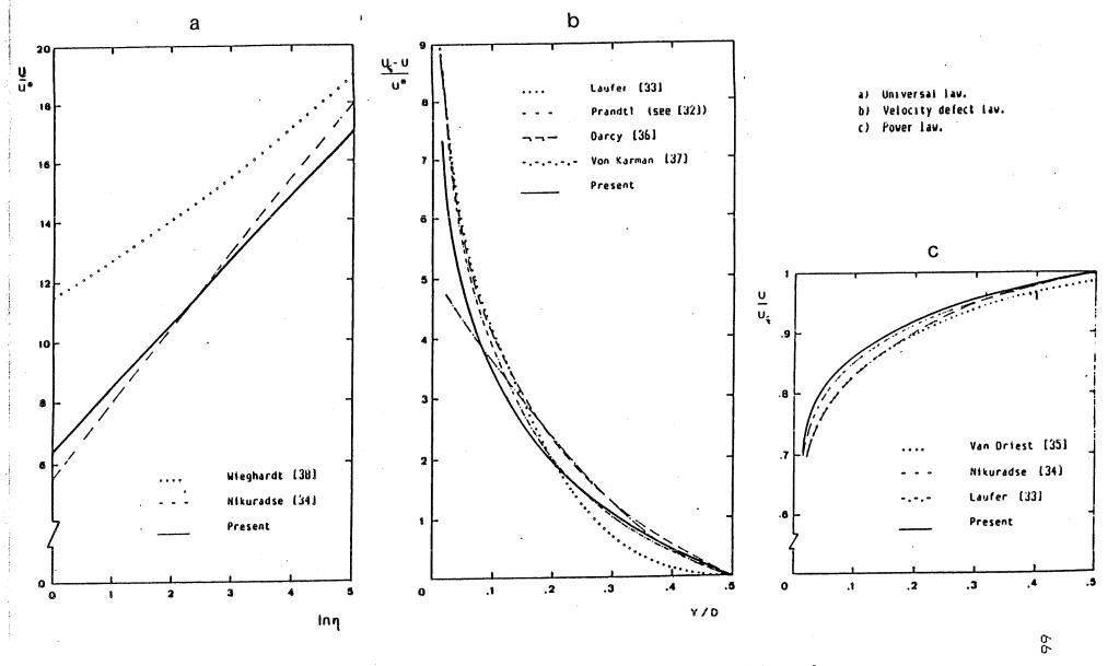
Figure 13 Verification of average velocity distribution laws in single phase flow.
