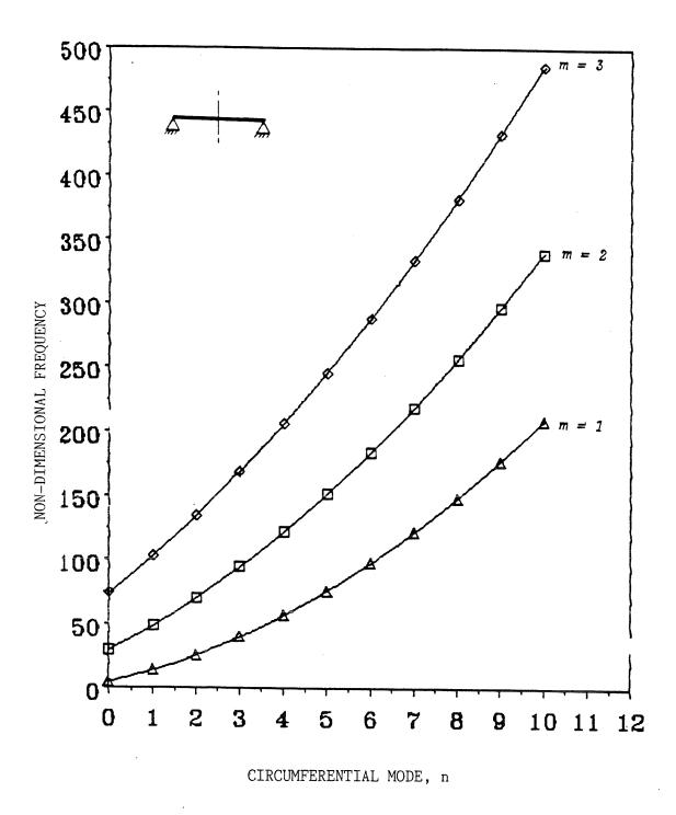
Figure 7.7: Non-dimensional natural frequency of a simply-supported circular plate as a function of the number of circumferential mode n.
