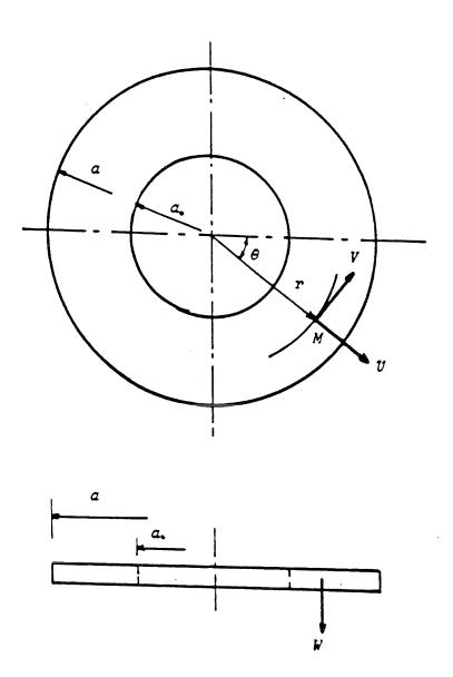
Figure 2.1: Geometry of the mean surface of a circular plate.
