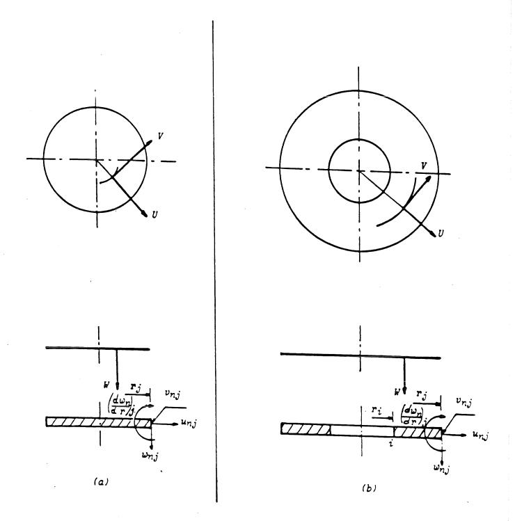
Figure 3.1: Displacements and degrees of freedom for one node
