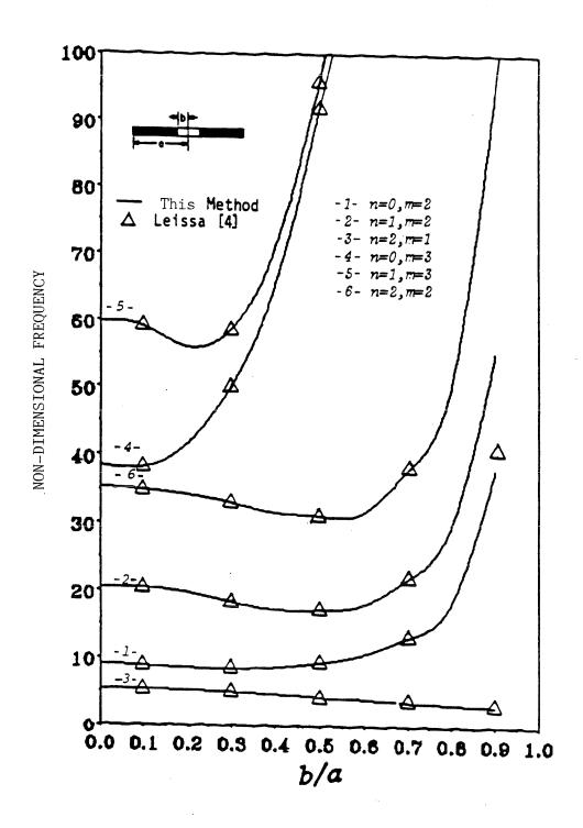
Figure 7.13: Non-dimensional natural frequency of a free-free plate.
