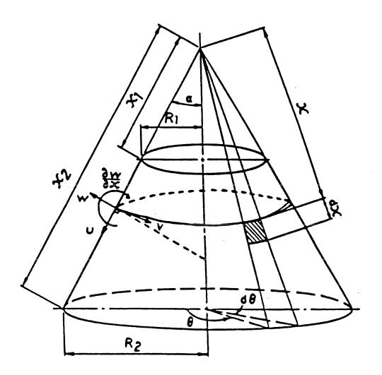
Figure A-1.2: Geometry of the mean surface of a conical shell.
