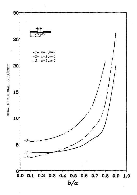
Figure 7.14: Non-dimensional natural frequency of a free - simply-supported plate.
