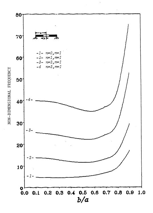
Figure 7.16: Non-dimensional natural frequency of a simply-supported - free plate.
