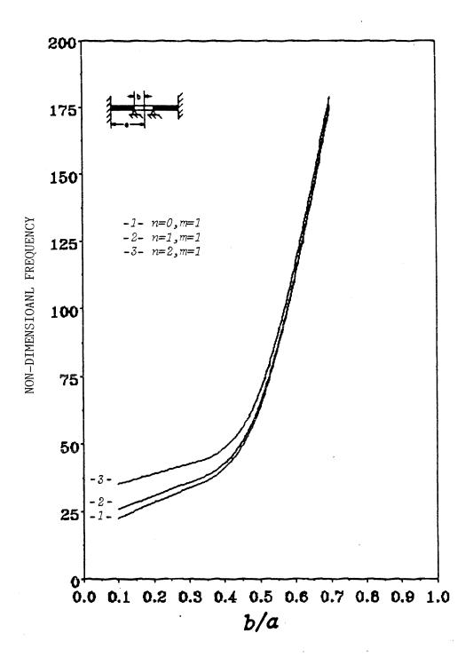
Figure 7.15: Non-dimensional natural frequency of a clamped - simply-supported plate.
