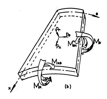
Figure A-1.1: Differential element for a conical shell
