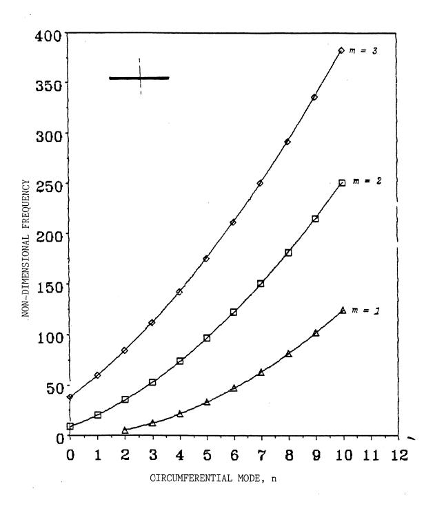
Figure 7.6: Non-dimensional natural frequency of a free circular plate as a function of the number of circumferential mode n.
