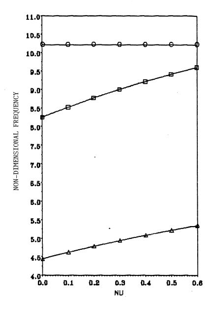
Figure 7.17: Non-dimensional natural frequency as a function of Poisson's ratio (n = 0, m = 1).
