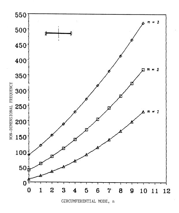
Figure 7.5: Non-dimensional natural frequency of a clamped circular plate as a function of the number of circumferential mode n.
