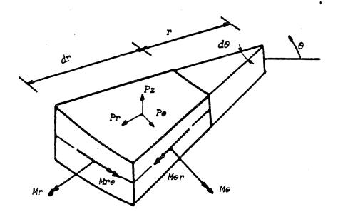
Figure 2.2: Differential element for a circular plate
