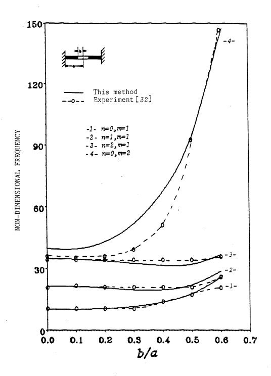
Figure 7.12: Non-dimensional natural frequency of a clamped-free plate.
