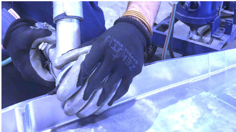
Figure 2.2 An operator manually peen forming a part. The operator uses a gloved hand to block part of the nozzle during the treatment. The flow of shot is kept constant and the operator's hand acts as a control shutter. Reproduced with permission from Aerosphère Inc.
