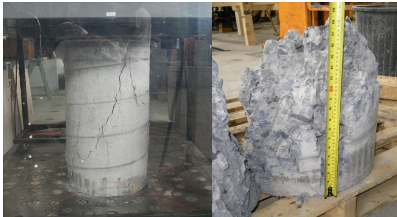
Figure 3-2: Mass concrete cylindrical specimen (400mm x 800mm)
