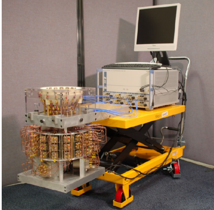
Figure 2.5 University of Bristol CMI clinical prototype. Image obtained from (Henriksson et al. (2011)).
