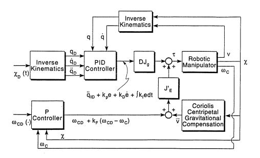
Figure 1: The Structure of the Motion/Force Controller
