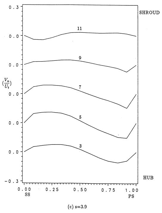
Figure 15: Blade-to-Blade Velocity Component  $V_n$ , Stator
