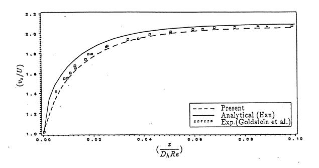
Figure 4: Center-Line Velocity Development,  $\gamma = 1.0$
