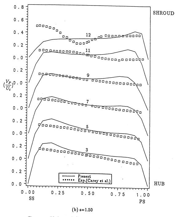
Figure 10: Blade-to-Blade Velocity Components  $V_p$ , Rotor
