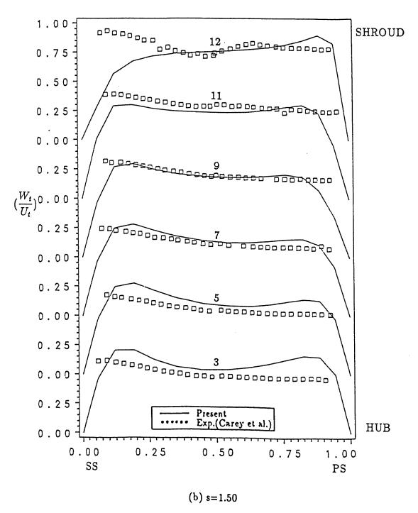
Figure 11: Blade-to-Blade Velocity Components  $W_t$ , Rotor
