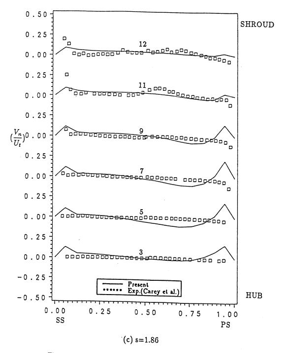
Figure 12: Blade-to-Blade Velocity Components  $V_n$ , Rotor
