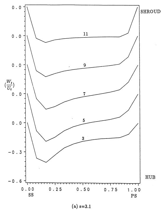
Figure 14: Blade-to-Blade Velocity Component  $V_t$ , Stator
