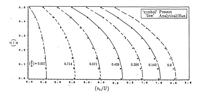
Figure 3: Fully-Developed Velocity Profiles,  $\gamma = 1.0$
