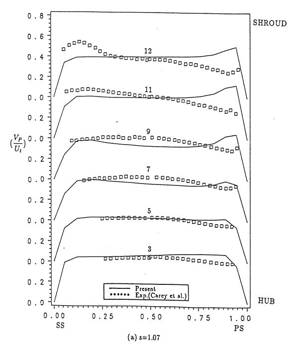
Figure 10: Blade-to-Blade Velocity Components  $V_p$ , Rotor
