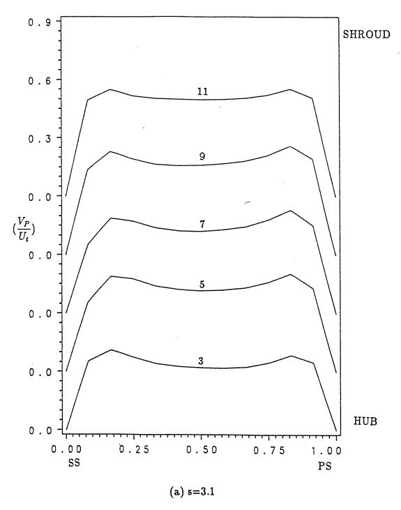
Figure 13: Blade-to-Blade Velocity Component  $V_p$ , Stator
