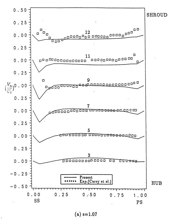
Figure 12: Blade-to-Blade Velocity Components  $V_n$ , Rotor
