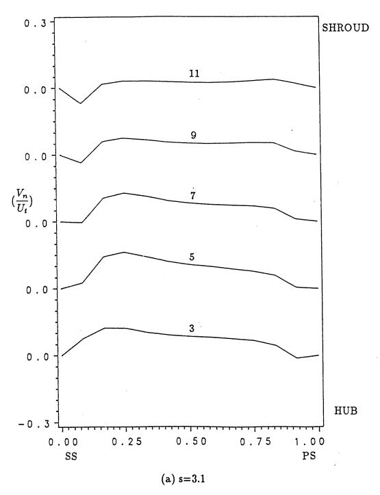
Figure 15: Blade-to-Blade Velocity Component  $V_n$ , Stator
