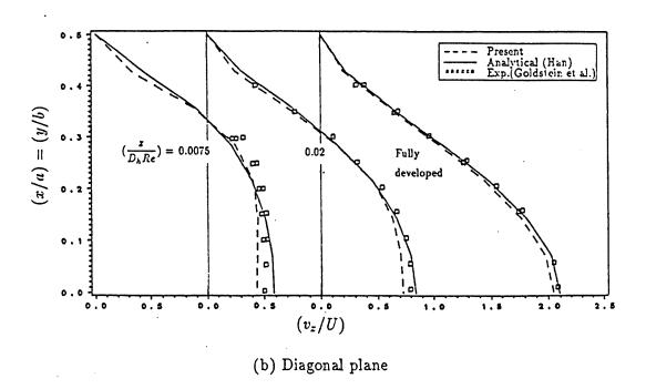
Figure 2: Velocity Development for a Straight Duct with Aspect Ratio  $\gamma=1.0$
