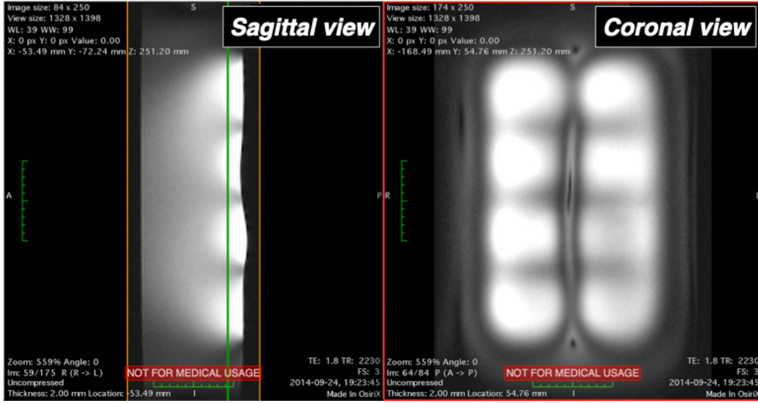
Figure 6.1: Magnitude images of rectangular water-filled box illustrating the inhomogeneous intensity artifacts resulting from the nonuniform B_1^+ profile of the custom 8-channel transceiver array. The problem is particularly evident as the darkened region in the middle of the coronal image (i.e. for a human subject, this is roughly where the spinal cord would be situated).
