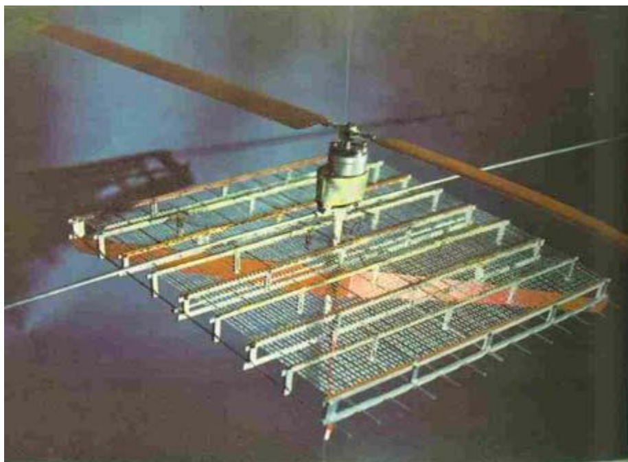
Figure 2.1 First microwave-powered helicopter built by W. C. Brown in 1964 [7]
