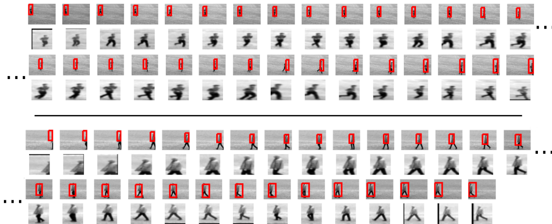
Figure 7.13 Two examples of tracking on the KTH data set. The layout for each example is as follows: the first row shows 15 frames of one test sequence with a red rectangle indicating the location of the glimpse. The second row contains the extracted glimpses. The third and fourth row show the continuation of the sequence. We only show every second frame.
